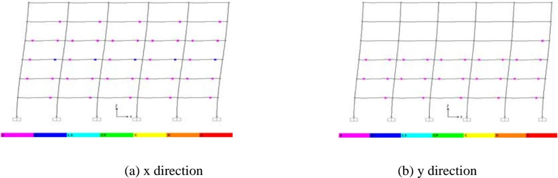
**Figure 4.2.** Status of plastic hinges of the 6 storey structure at the end of the pushover analysis under the triangular loading
