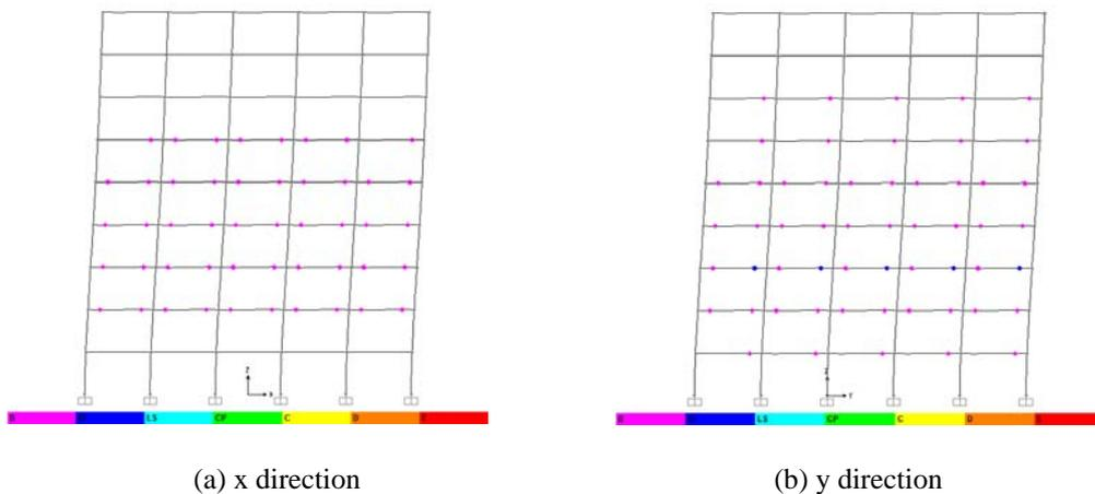
**Figure 4.5.** Status of plastic hinges of the 9 storey structure at the end of the pushover analysis under the rectangular loading
