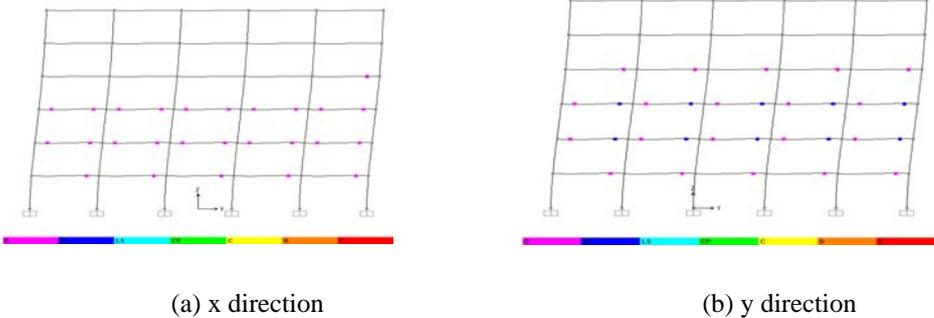
**Figure 4.3.** Status of plastic hinges of the 6 storey structure at the end of the pushover analysis under the rectangular loading
