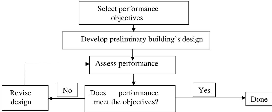
**Figure1.1** Performance-based design flowchart (FEMA 445-B, 2006)
