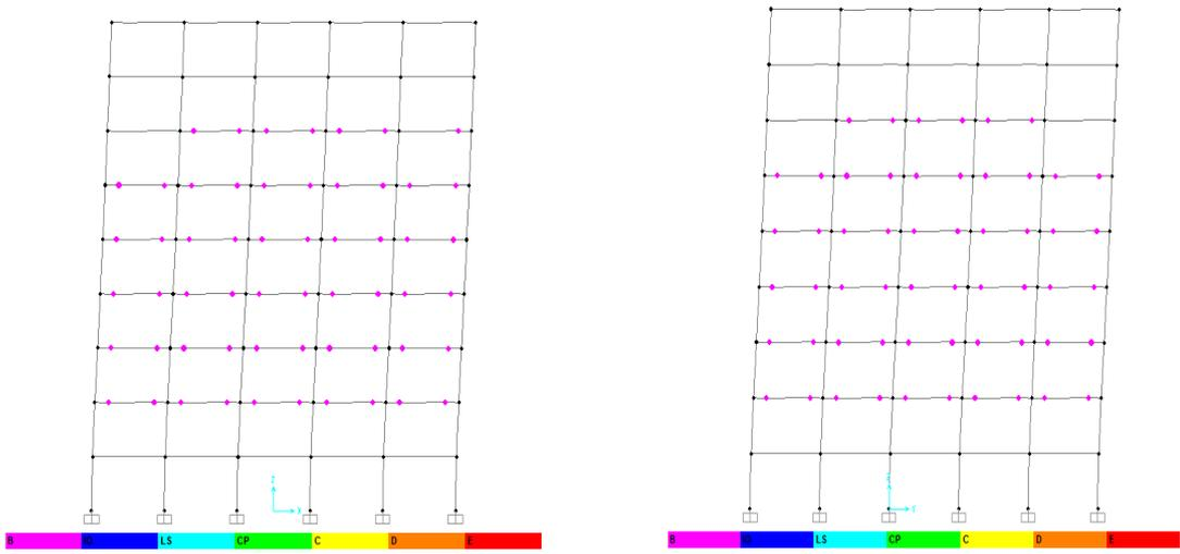
**Figure 5.5.** Status of plastic hinges of the 9 storey structure at the end of the pushover analysis under the triangular loading
