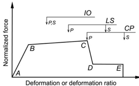
**Figure 4.1-** Behavior and performance limits in a typical hinge (FEMA 356, 2000)
