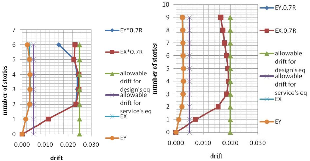
Figure 3.1- Drift angle of the structures against the service and the design level earthquakes
