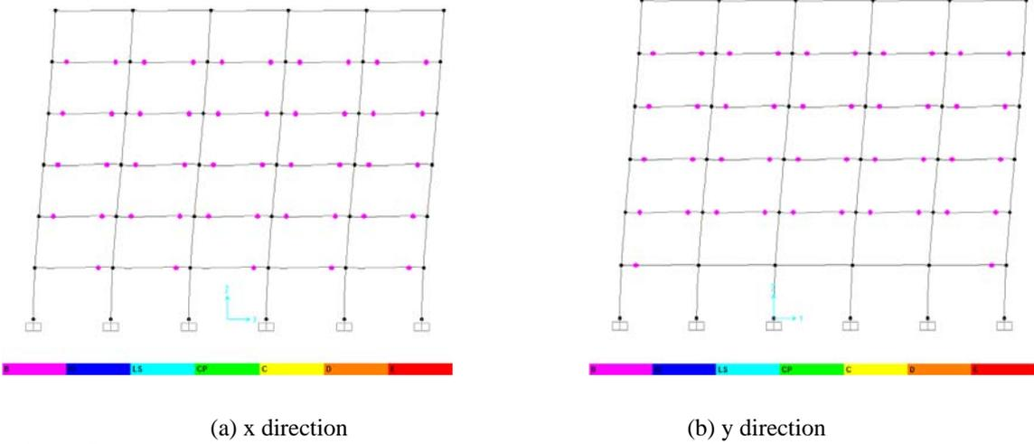
**Figure 5.1.** Status of plastic hinges of the 6 storey structure at the end of the pushover analysis under the triangular loading
