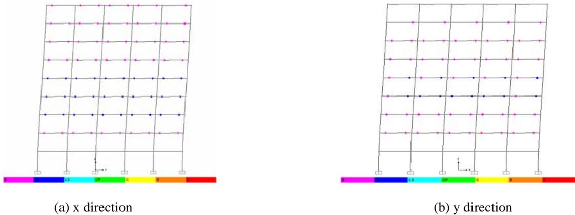
**Figure 4.4.** Status of plastic hinges of the 9 storey structure at the end of the pushover analysis under the triangular loading
