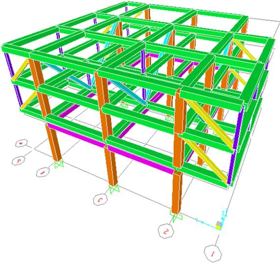
**Figure 2.3.** A 3D View of the Structural Model with tie-Beams (purple colour elements) in SAP2000.
