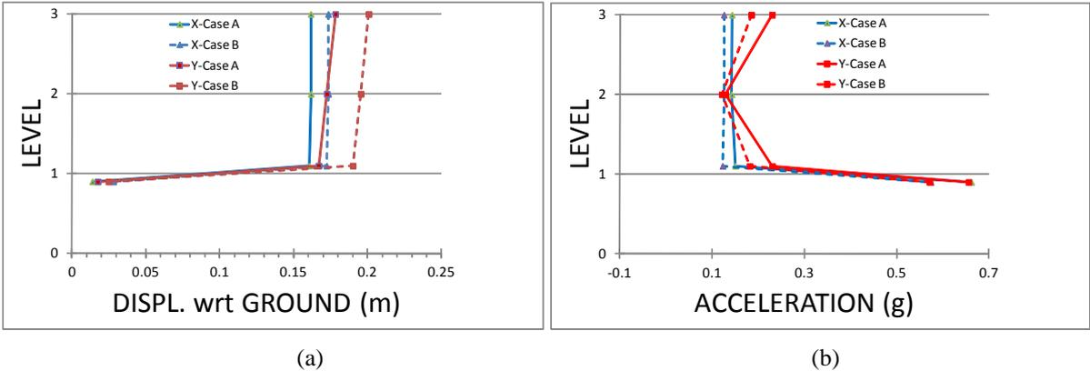
Figure 4.1. Average (a) Floor/Level Displacements, and (b) Level Accelerations.
