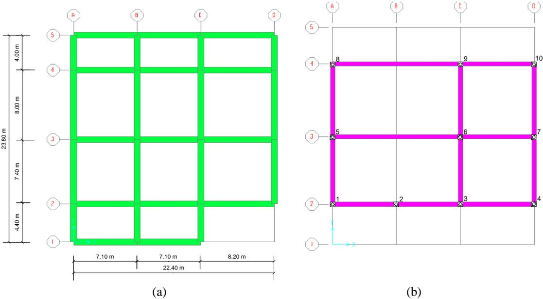
**Figure 2.1.** Plan view of (a) the building floors and (b) the Isolation Interface with the Grid of the tie-Beams of the Basement Columns.
