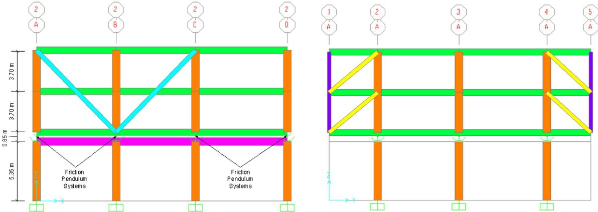
**Figure 2.2.** Side Views of (a) the Grid Line #2 of Case A with the Tie-Beams (Pink) on the Basement Column Tops, and (b) the Grid Line #A of Case B without Tie-Beams.
