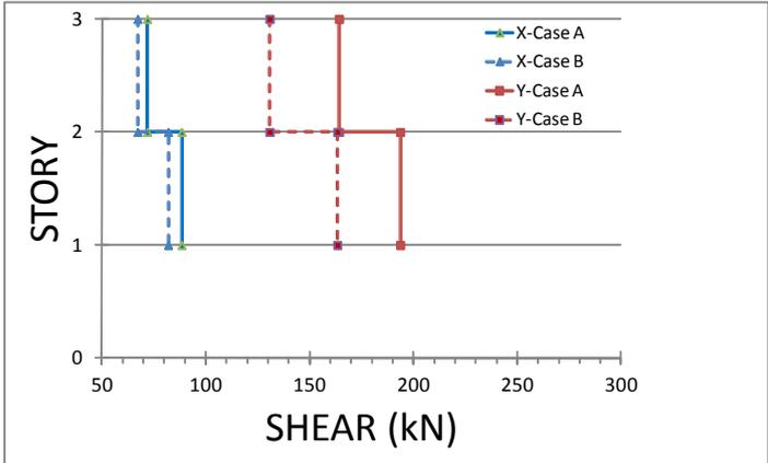
Figure 4.2. Average (over 20 motions) shear for Column 2-A directly above Isolator #1.
