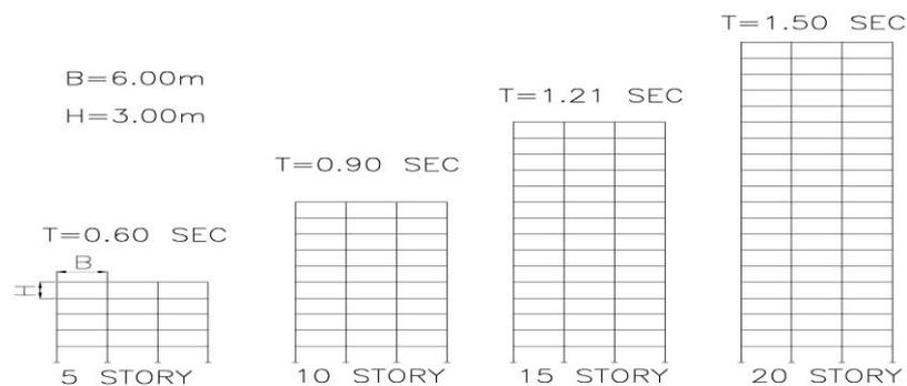
**Figure 3.** Test frames in analysis
