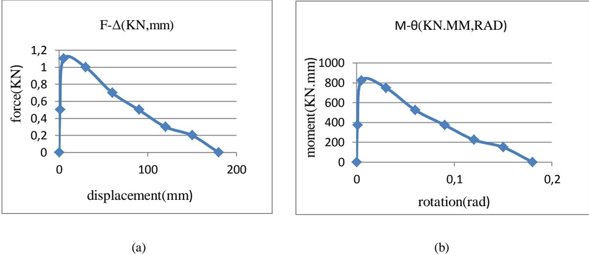
Figure 2. Bending plastic hinge behavior diagram: a).Force-displacement; b) Moment-rotation
