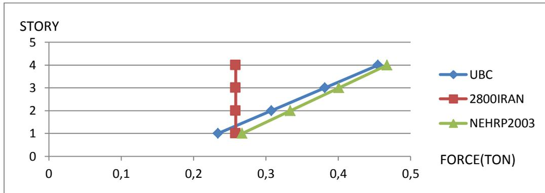
Figure 10. Loads to Masonry Walls in Standards
