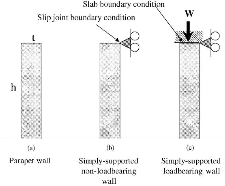
Figure 1. Unreinforced masonry wall support configurations
