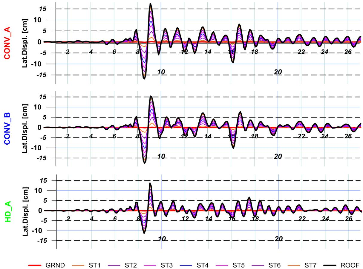
Figure 6. Story displacement time-history of all three models under Izmit earthquake, X direction
