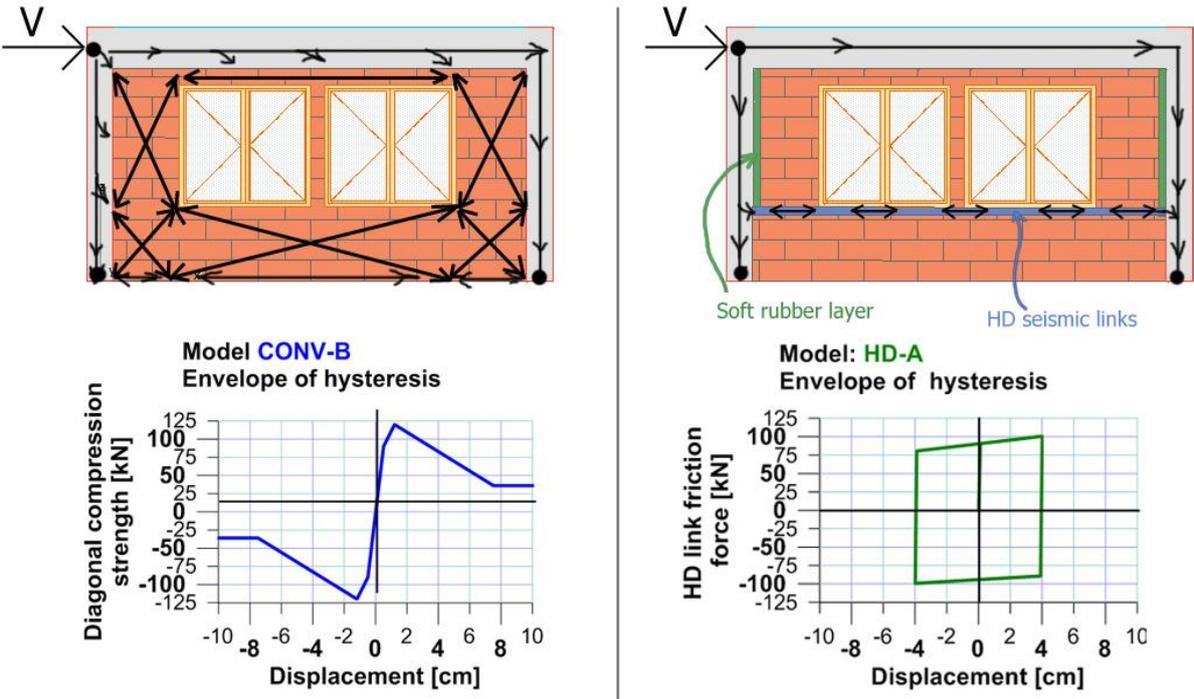
Figure 4. Response mechanism of conventional and HD infill wall panels
