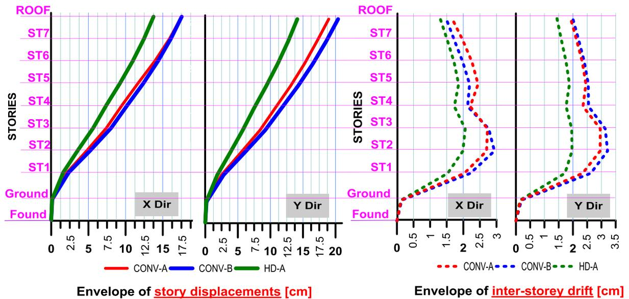
Figure 7. Envelopes of story displacements and drifts in X and Y dir, under Izmit earthquake
