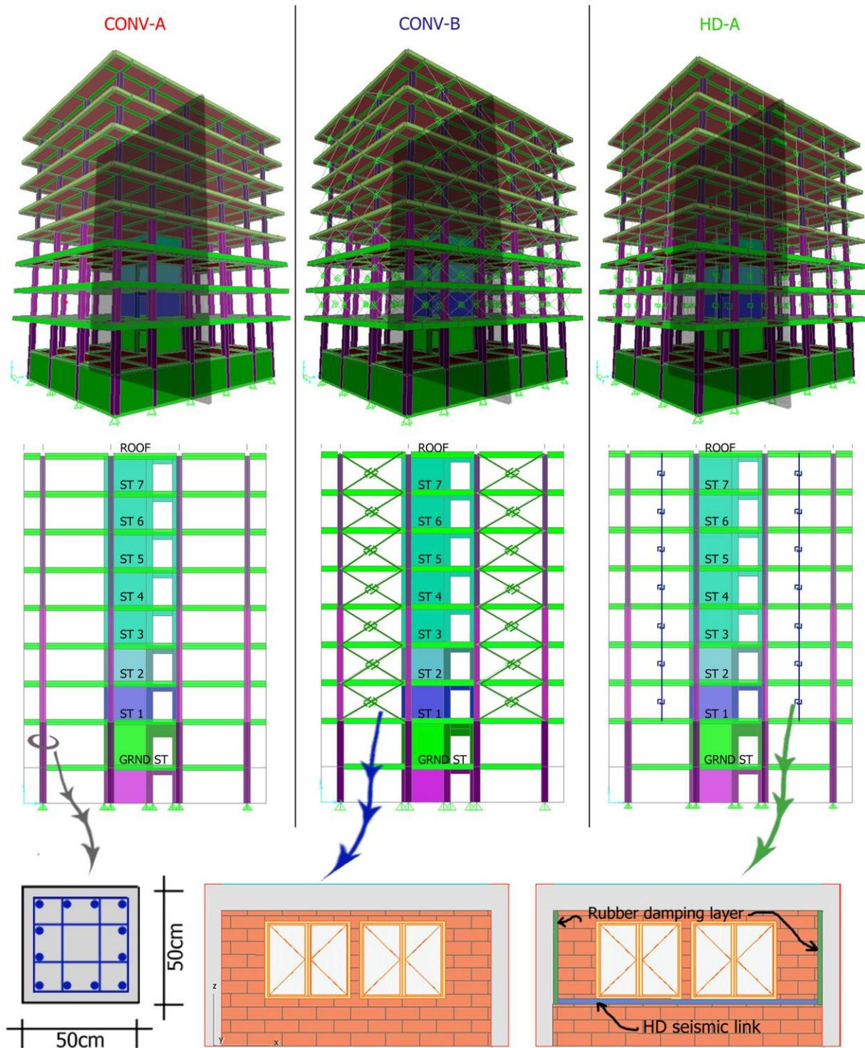
**Figure 3.** 3D mathematical models representative for the 7 storey building constructed in Shkup, Macedonia
