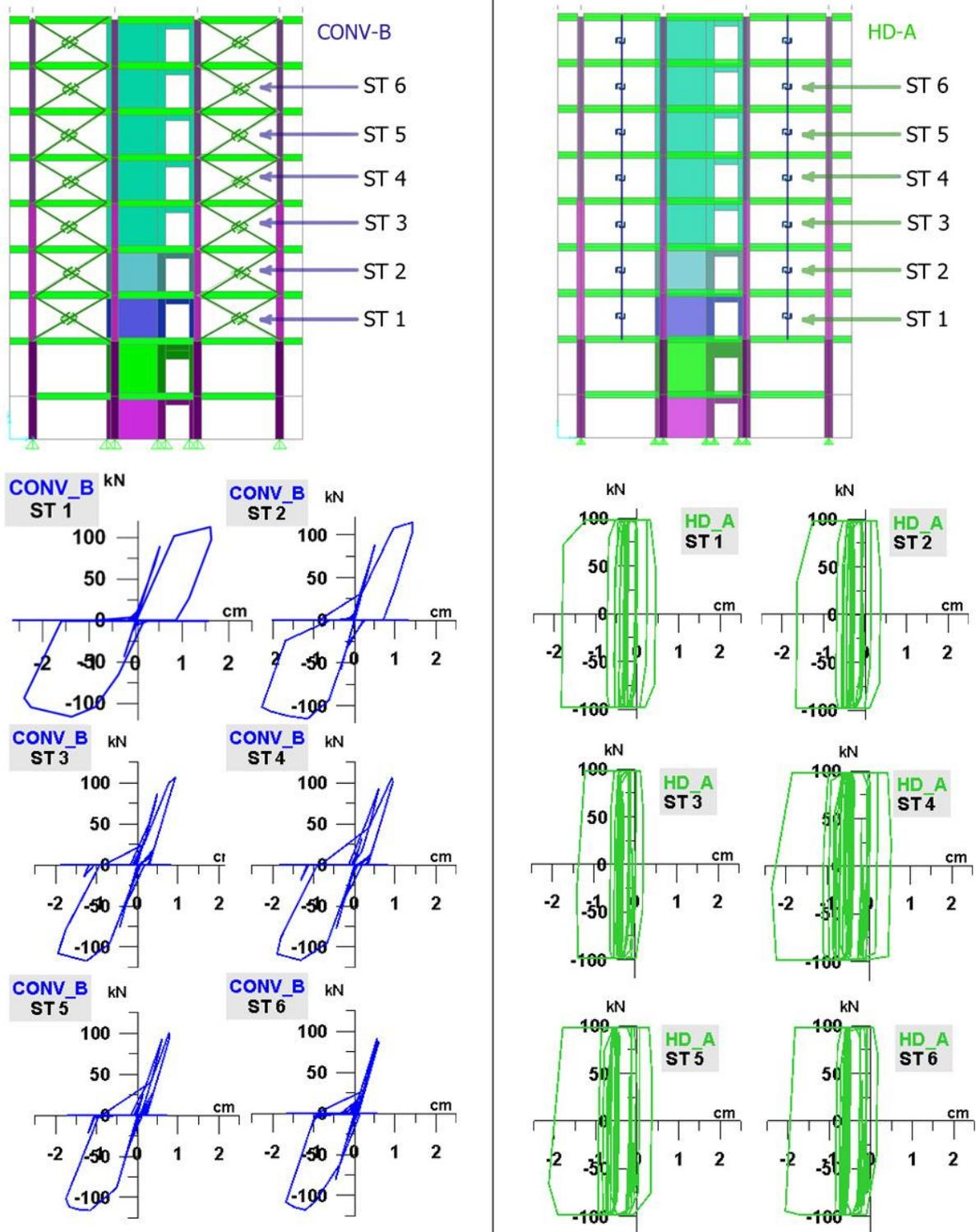
**Figure 8.** Hysteretic behavior of infill panel element, under Izmit earthquake - X direction
