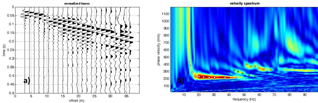
**Figure 3.** Multichannel shot record a) Frequency - Phase Velocity spectra with fundamental mode picking, and two additionally picked higher modes.
