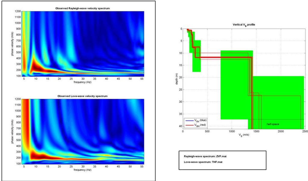
**Figure 7.** Inverted  $V_s$  section, from site 2 in figure 2, with a resulting  $V_s^{30}$  value of 417 m/s.
