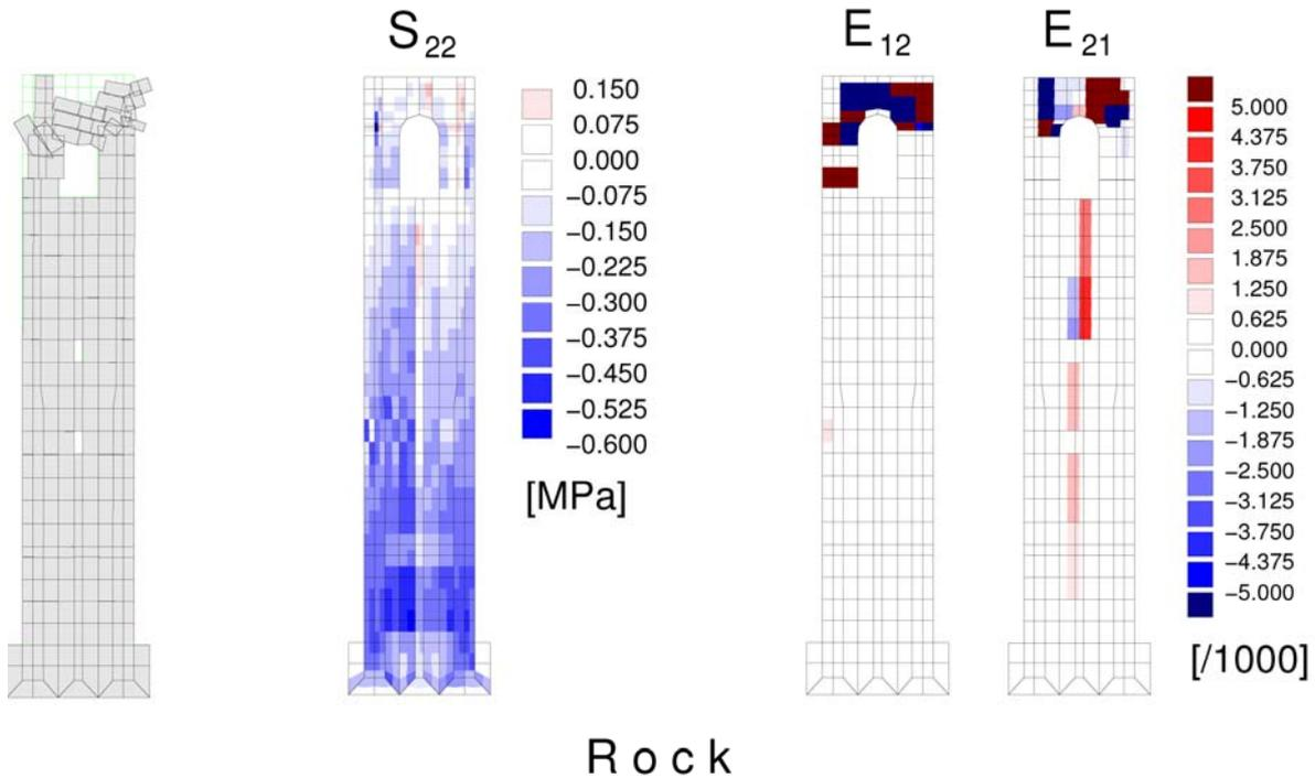
**Figure 9** Results of the non linear dynamic analyses for the scheme 1– rock soil. From left to right: final deformed shape; map of the shear deformation  $E_{12}$  and  $E_{21}$ ; map of the  $S_{22}$  stress component.
