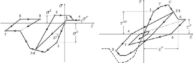
**Figure 2.** Scheme of the hysteretic rules for the axial (left), and shear springs (right).
