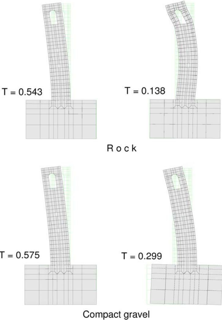
Figure 6 The first 2 mode shapes in the presence of a rock soil and compact gravel soil.
