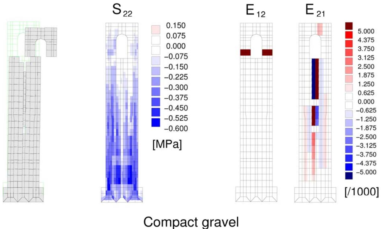
**Figure 10** Results of the non linear dynamic analyses for the scheme 2 – compact gravel soil. From left to right: final deformed shape; map of the shear deformation  $E_{12}$  and  $E_{21}$ ; map of the  $S_{22}$  stress component.
