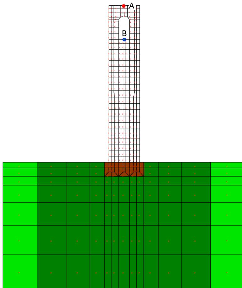
**Figure 5** Mesh of the tower with the significant volume of soil included in the model, and location of the control points A and B.
