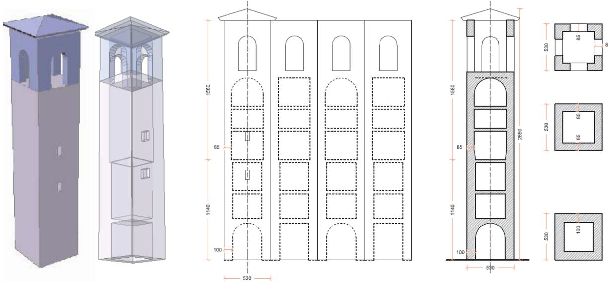
**Figure 4.** 3D drawing, schematic prospects, section and plan views of the idealized case study.
