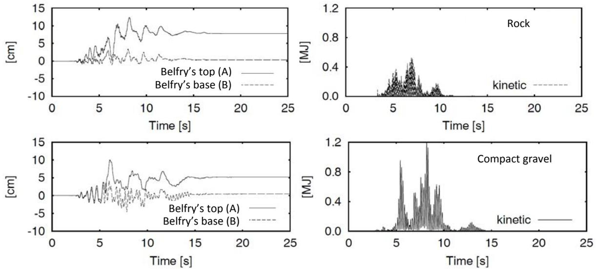
**Figure 8** Displacement time history (left) for the control points (see Fig. 5) and kinetic energy (right).
