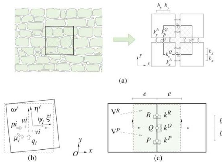
**Figure 1.** Scheme of the RVE in relation with the unit cell defined by 4 rigid elements (a); kinematics (b); disposition of the connecting spring-devices (c) (Casolo, 2004).
