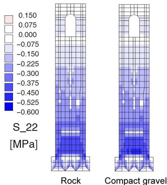
**Figure 7** Map of the vertical axial stress component  $S_{22}$  for the two schemes.
