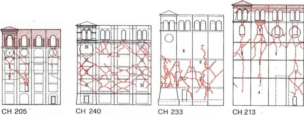
**Figure 3** Some typical geometry and damage patterns of Italian bell-towers (Doglioni et al., 1994).
