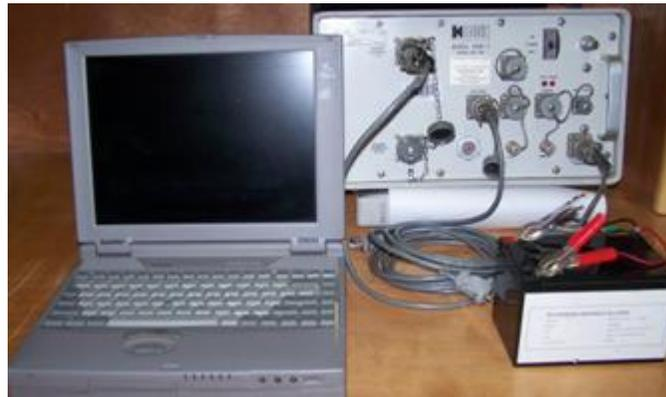
**Figure 1.4.** Recorder and laptop for the capture of information of vibration
