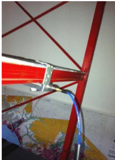
**Figure 2.6.** Photograph of the accelerometer placed in the structure.
