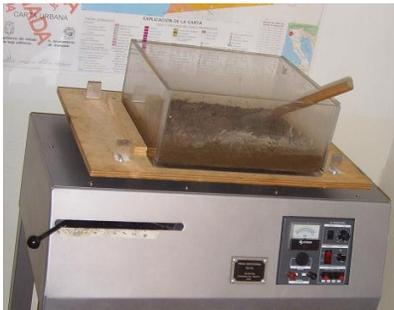
**Figure 2.9.** Photograph of the sample on the shake table.
