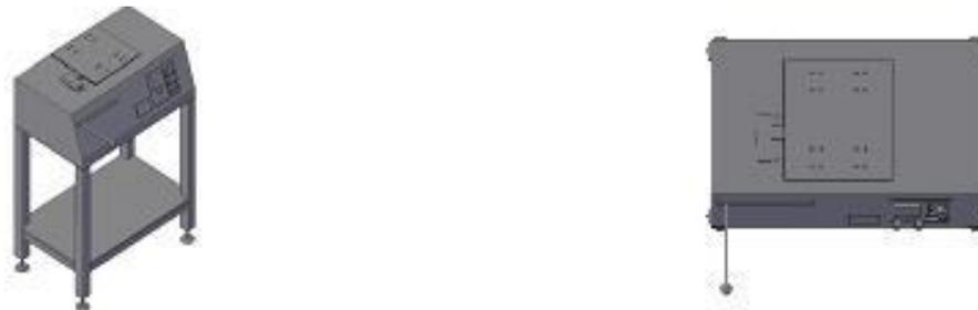
**Figure 1.1.** Shake Table. Left side an isometric, and to the right plant view.
