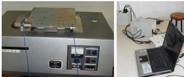
**Figure 1.2.** In the photograph of left three accelerometers connected to the table, and in the photograph of the right the regulator of voltage, the signal conditioner and the laptop.
