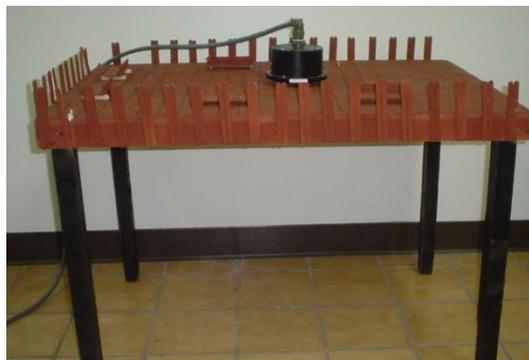
**Figure 2.2.** Structure used to measure vibration. The accelerometer is placed in the center.
