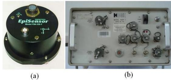
**Figure 1.3.** (a) Accelerometer Episensor Model FBA ES-T and (b) 16 bits Recorder.
