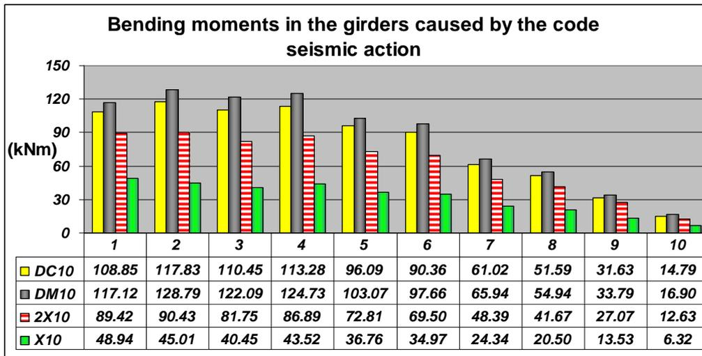
Figure 7. Bending moments in the girders caused by the horizontal seismic action
