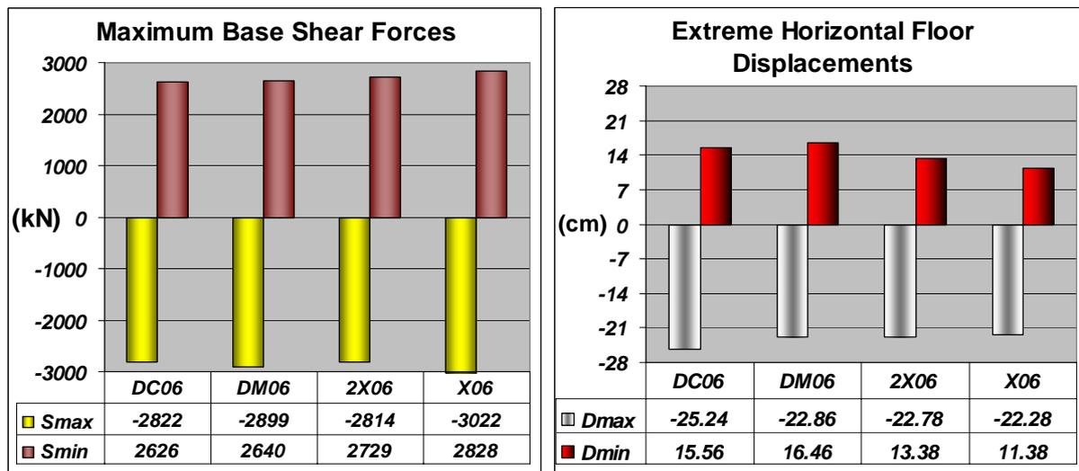
Figure 8. Extreme values for base shear forces and horizontal floor displacements recorded during the dynamic nonlinear analyses
