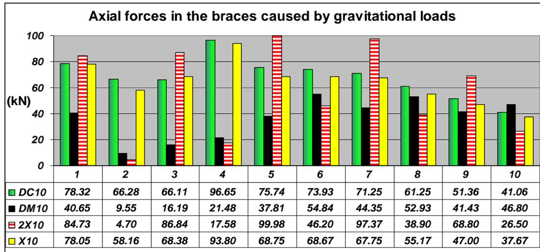
**Figure 6.** Compression forces in the braces caused by gravitational loads
