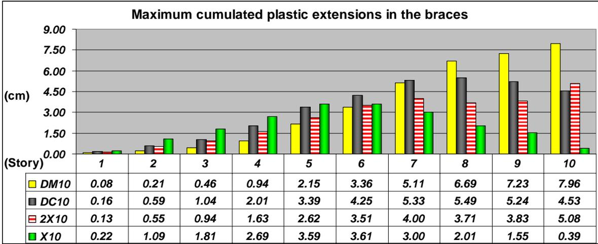
Figure 10. Maximum cumulated inelastic lengthening of the braces recorded after the dynamic nonlinear analyses
