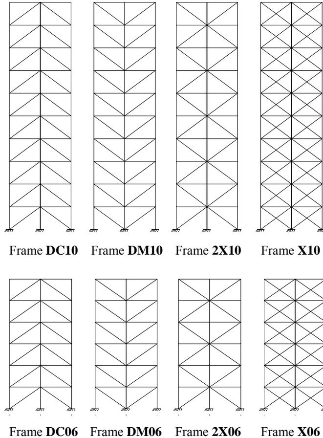
**Figure 1.** Analyzed diagonal braced frames
