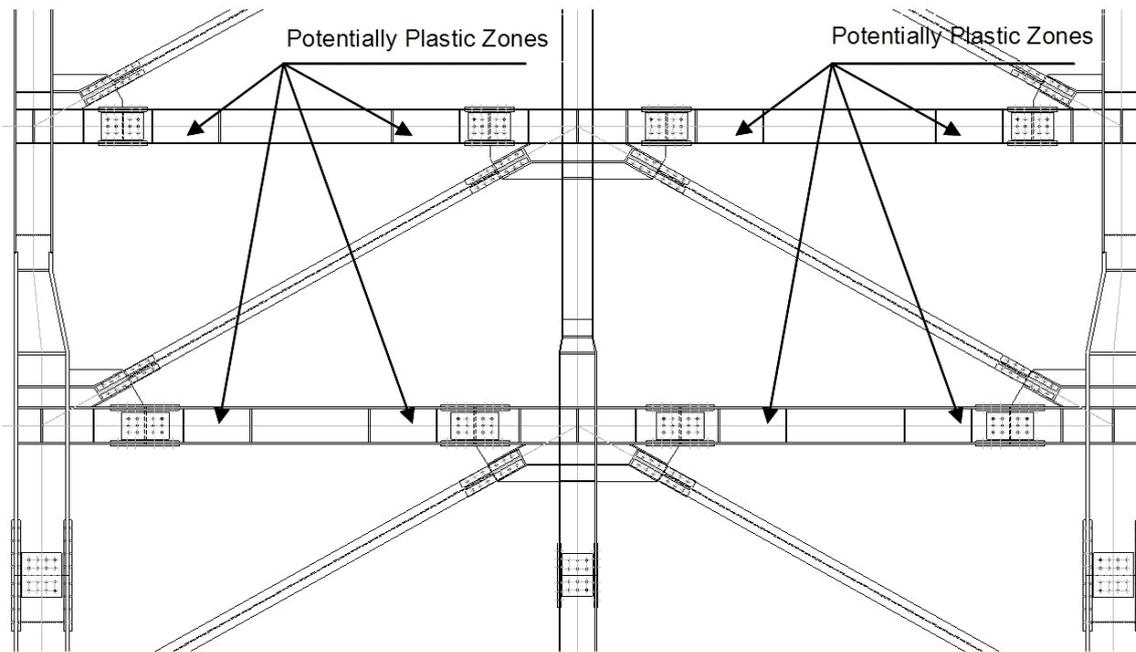
**Figure 2.** Location of the potentially plastic zones in the girders of a braced frame
