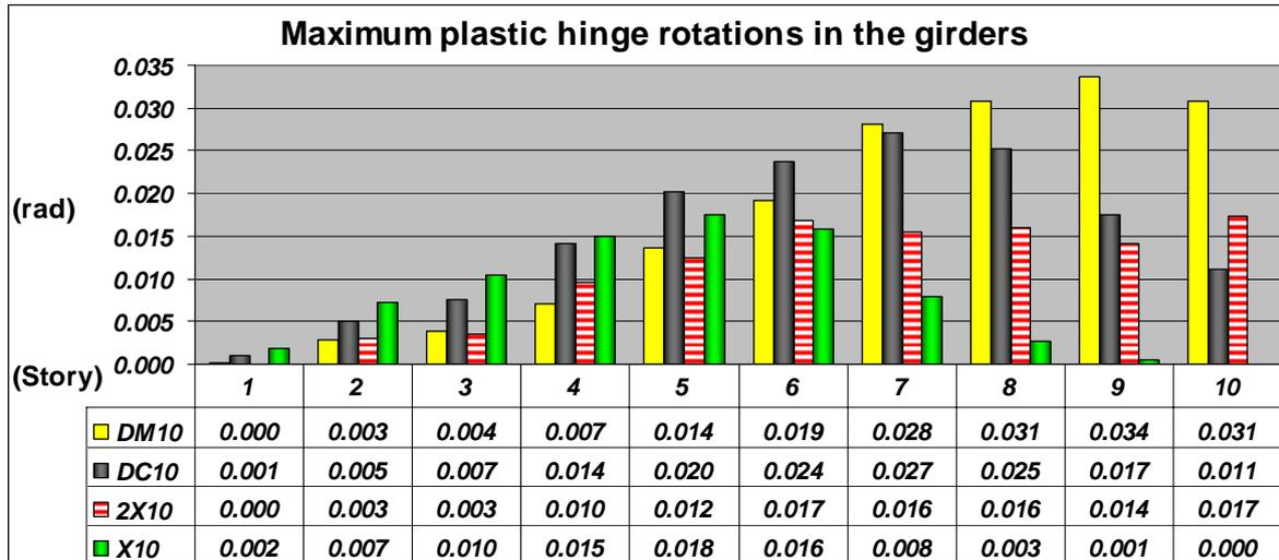
**Figure 11.** Maximum plastic hinge rotations in the girders recorded during the dynamic nonlinear analyses
