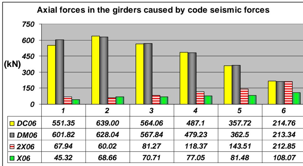
**Figure 5.** Axial forces in the girders generated by the horizontal seismic action
