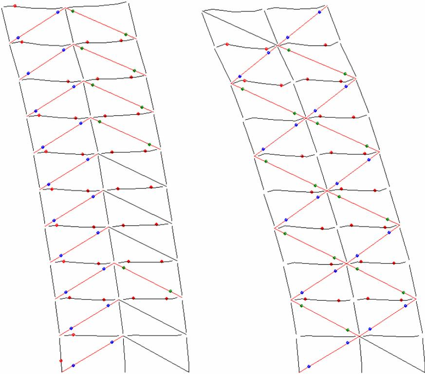
Figure 9. Plastic hinge distributions at 7.02 seconds from the start of the dynamic nonlinear analyses
