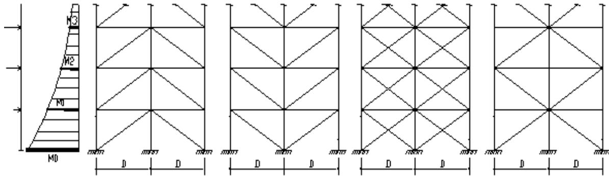
**Figure 3.** Lateral column axial forces caused by the horizontal seismic action
