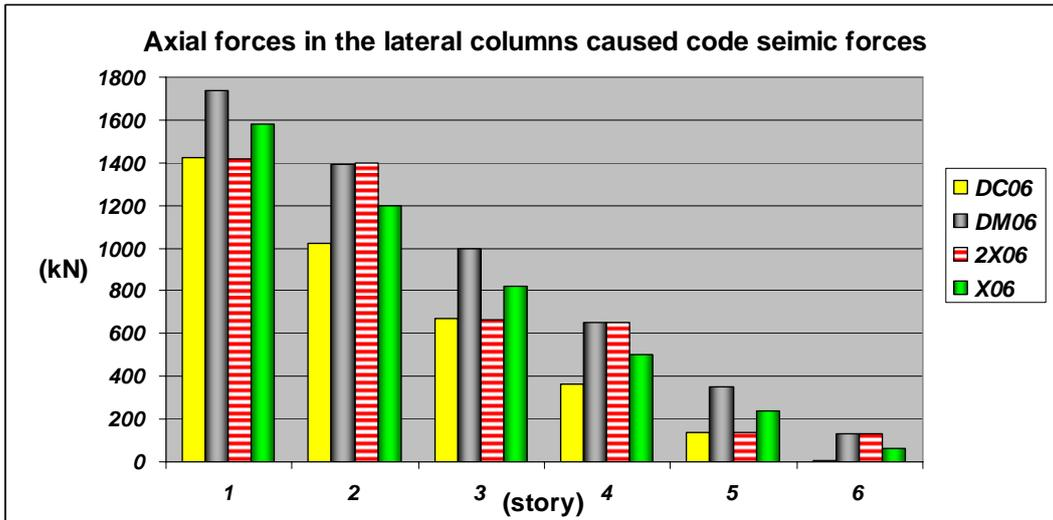
**Figure 4.** Axial forces in the lateral columns produced by code seismic forces
