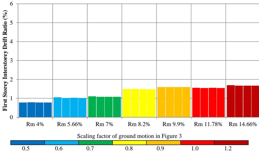
Figure 6. Lateral resistance (%W) required to surviving shaking sequence vs. interstorey drift ratio.
