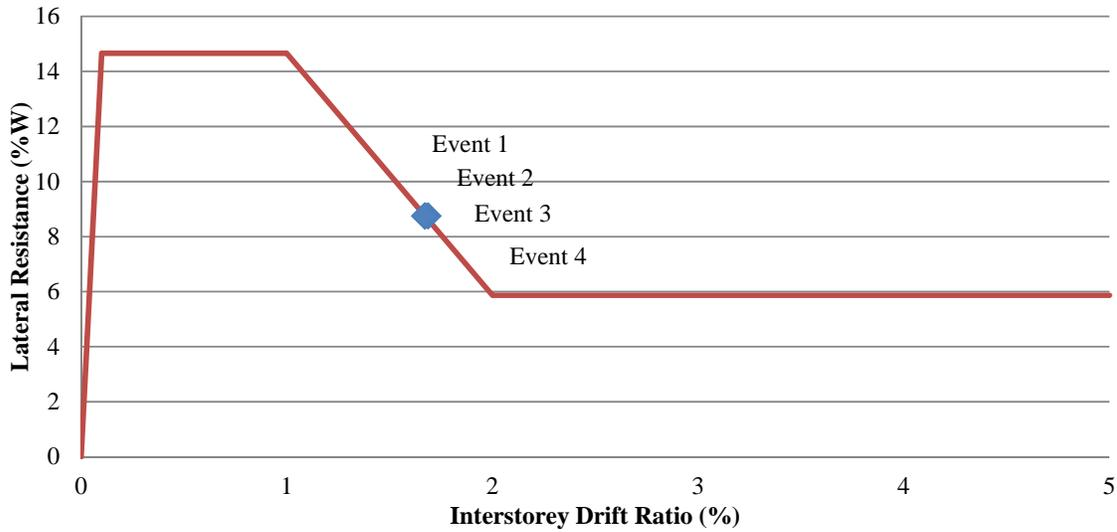
Figure 5. Sequence of first storey peak interstorey drift ratio on backbone curve for P= 14.66%W.
