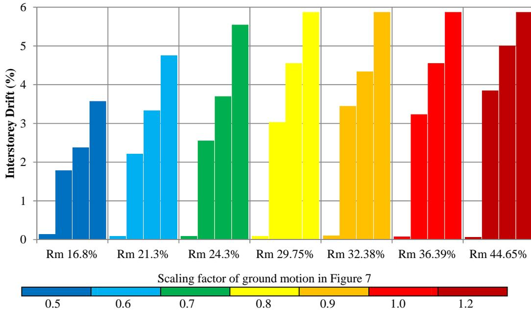
**Figure 10.** Lateral resistance (%W) required to surviving shaking sequence vs. interstorey drift ratio.
