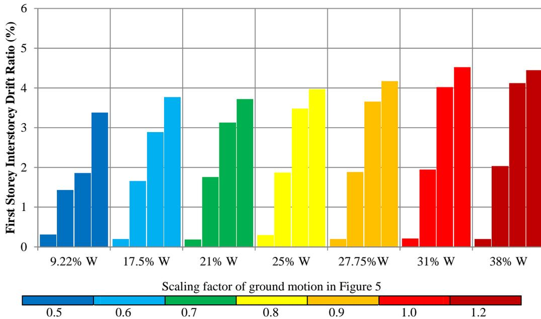
**Figure 8.** Lateral resistance (%W) required to surviving shaking sequence vs. interstorey drift ratio.
