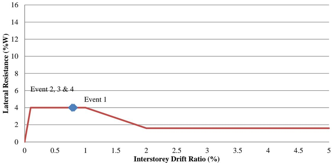
**Figure 4.** Sequence of first storey peak interstorey drift ratio on backbone curve for P= 4.0%W.
