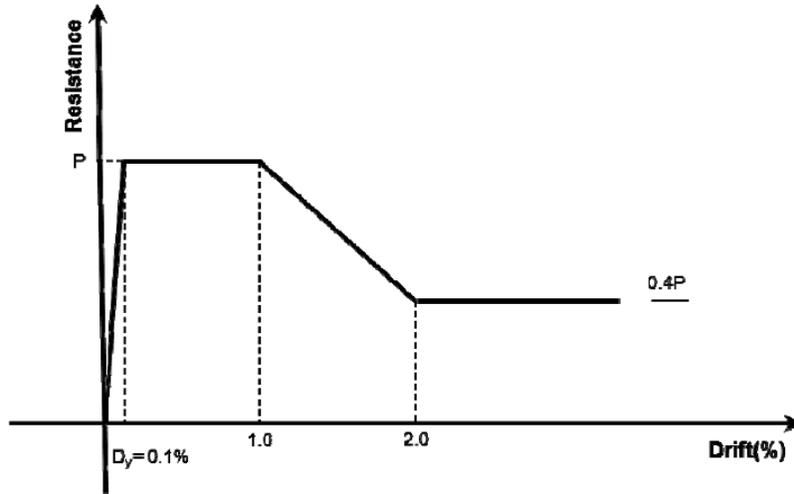
Figure 2. Squat RC shear wall backbone curve.
