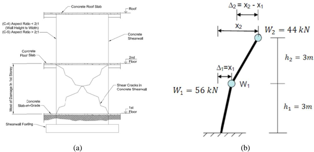
Figure 1. Squat RC shear wall prototype and stick model representation.
