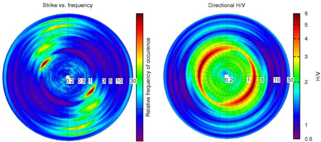
**Figure 3.1:** Comparison of two processing methods of single station three-component ambient vibration measurements. The relative occurrence of strike (azimuth) of ambient vibrations obtained with time-frequency polarization analysis is presented at left. The directional dependent H/V ratio is presented on right. Frequency changes along the radius from 0.2 to 30 Hz as indicated.
