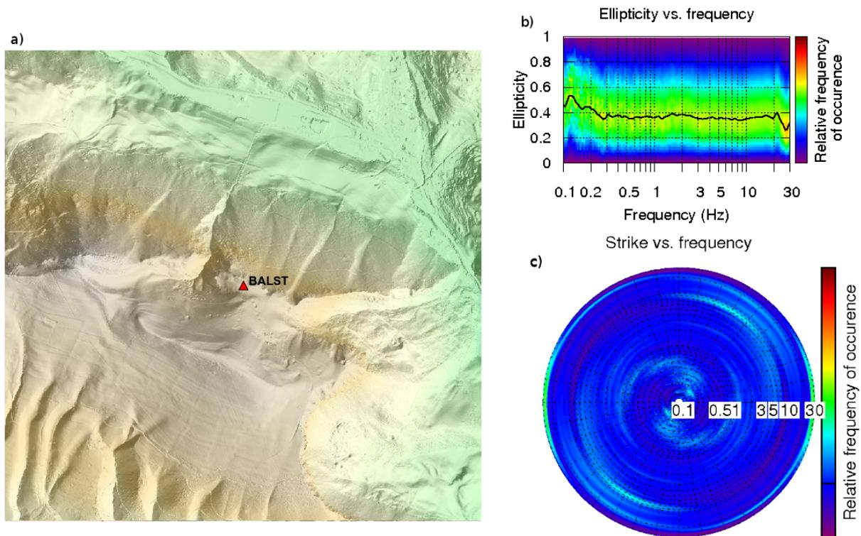
**Figure 4.3:** a) Site BALST (+ surrounding area of 2 km x 2 km), the height of the ridge is approximately 300 m. b) Relative frequency of occurrence of ellipticity in ambient vibrations retrieved by TFPA. The mode of the ellipticity distribution is interconnected with the black line; c) Relative frequency of occurrence of strike in ambient vibrations retrieved by TFPA.
