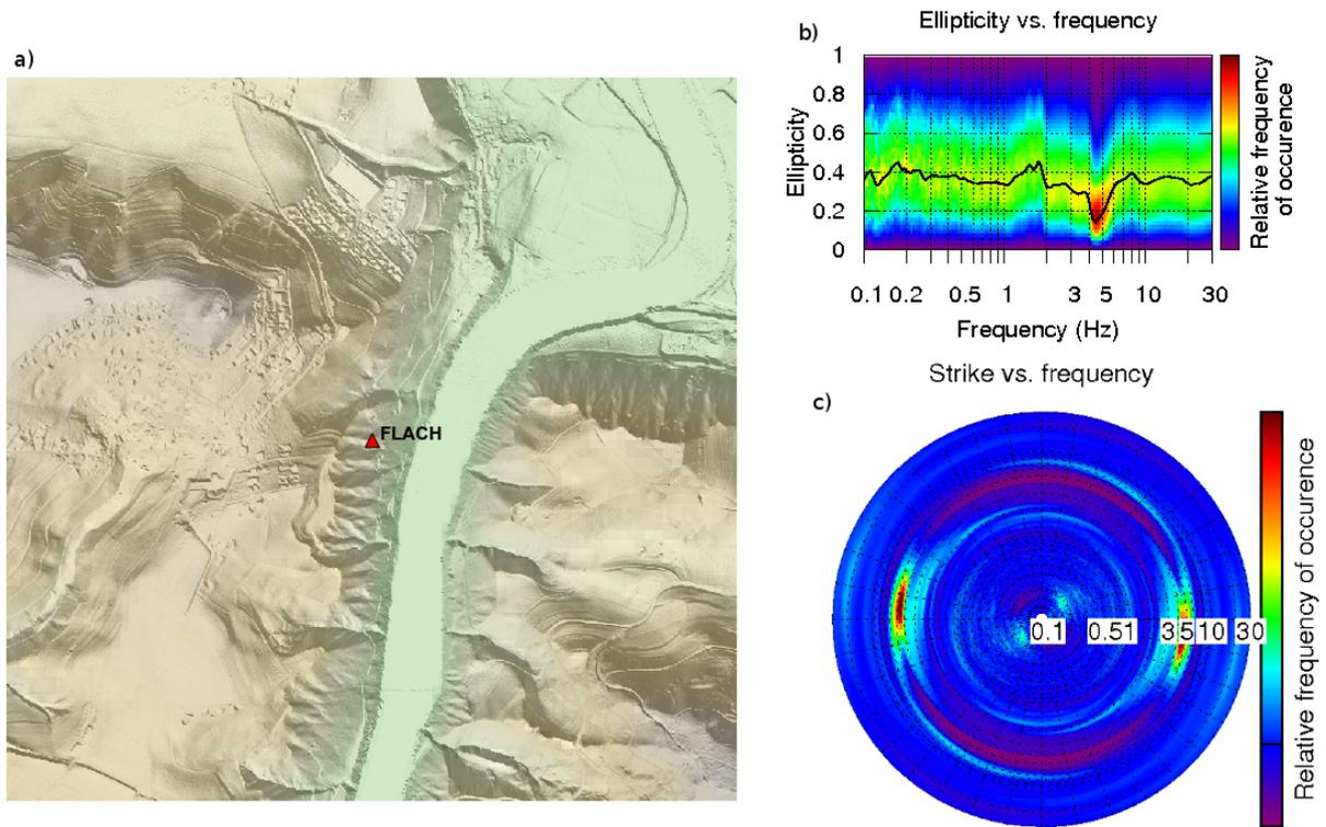
**Figure 4.1:** a) Site FLACH (+ surrounding area of 2 km x 2 km), the height of the ridge is approximately 150 m. b) Relative frequency of occurrence of ellipticity in ambient vibrations retrieved by TFPA. The mode of the ellipticity distribution is interconnected with the black line; c) Relative frequency of occurrence of strike in ambient vibrations retrieved by TFPA.
