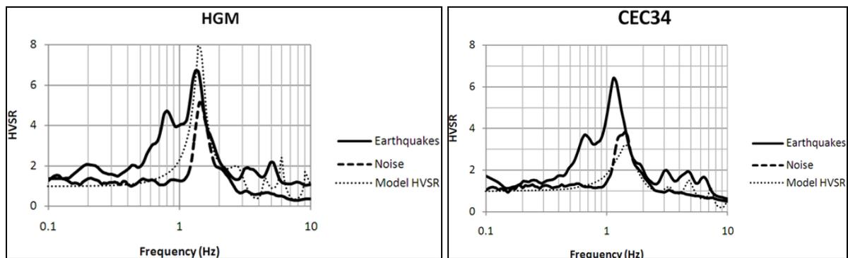
**Figure 3.** HVSR curves obtained from records of earthquakes, microtremor and a theoretical model for two recording sites in the study area
