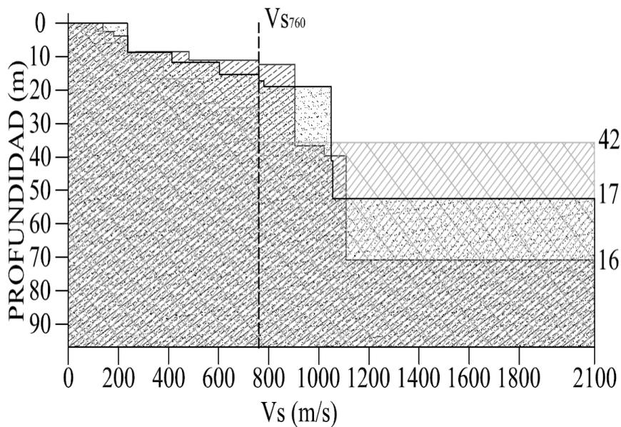
**Figure 8.** Vs wave velocities estimated with the ModelHVSR using the microtremor records of the sites 16, 17 and 42
