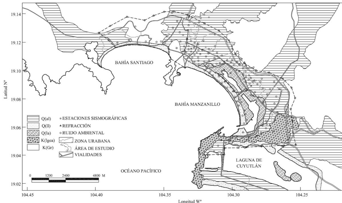
**Figure 2.** Indicates the study area boundary. Circles show the microtremor recording points, triangles define multichannel seismic refraction and squares the location of temporarily seismic station
