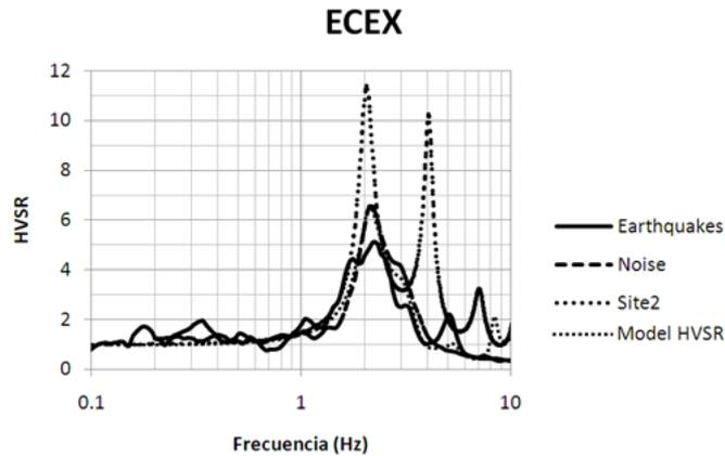
**Figure 4.** HVRS curves obtained from records of earthquake, microtremor, seismic refraction and a theoretical model for the ECEX site
