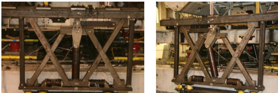
**Figure 2.1.** Views of Negative Stiffness Device [(a): Un-deformed NSD; (b): Deformed NSD]
