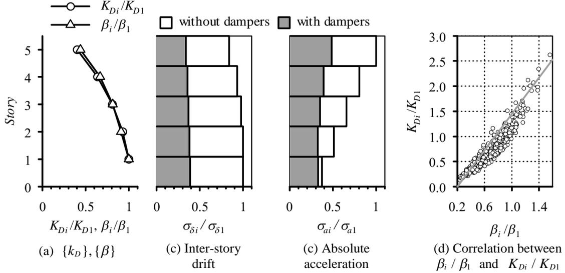
**Figure 3.** Distribution of optimal dampers and their effect on inter-story drifts and absolute accelerations
