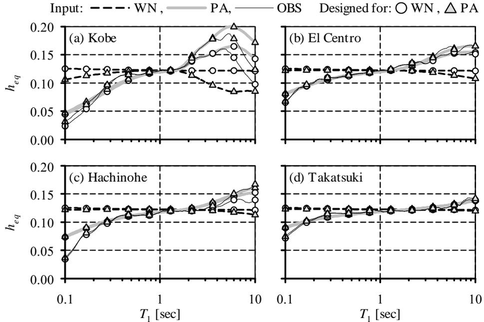
**Figure 5.** Equivalent damping factors for three types of input ground motion models
