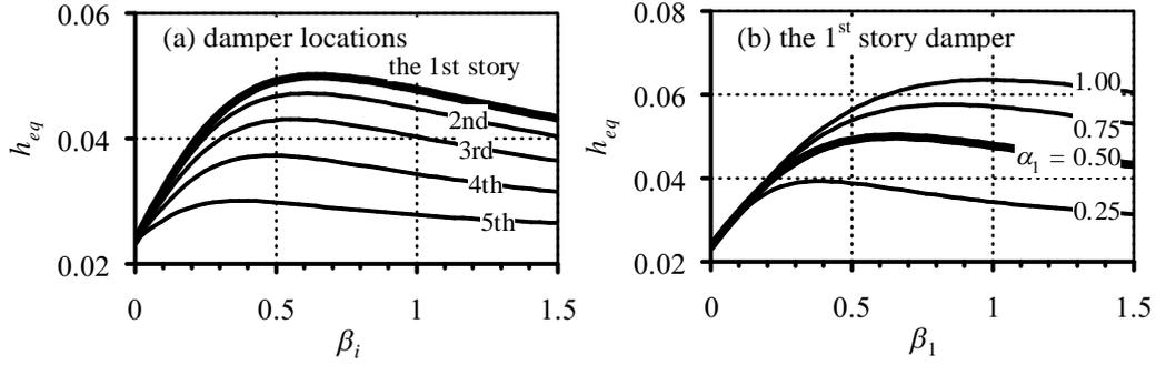
**Figure 2.** Dependence of equivalent damping factor on non-dimensional damping coefficient
