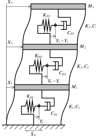
**Figure 1.**  $N$ -story structural model with Maxwell dampers
