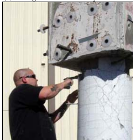
(c) Hammer test to remove loose material
