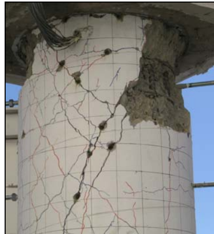
(b) Damage state of as-built specimen SP2
