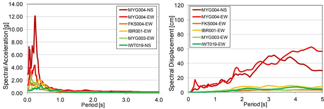
**Figure 3.1** Comparison of 5% damped elastic response spectra computed from six EQGMs recorded during the 2011 Tohoku earthquake: (a) Acceleration response spectra; (b) Displacement response spectra.
