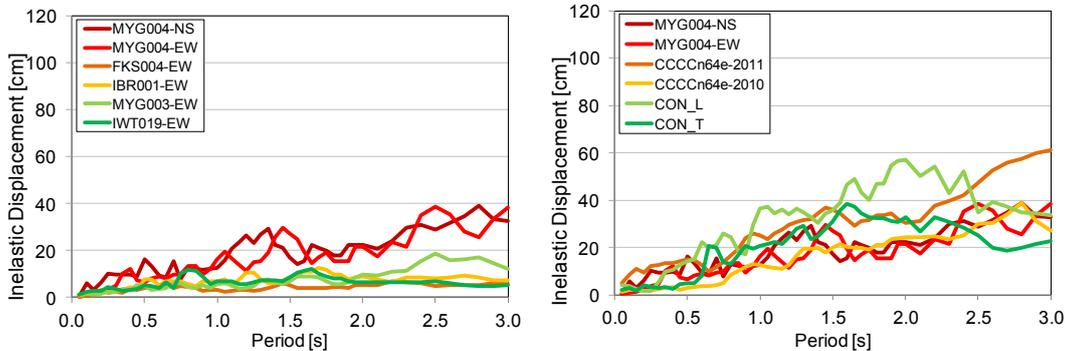
**Figure 5.2.** Inelastic displacement spectra for the selected earthquake ground motions ( $R=3$ ): a) Selected Japanese records, b) selected EQGMs
