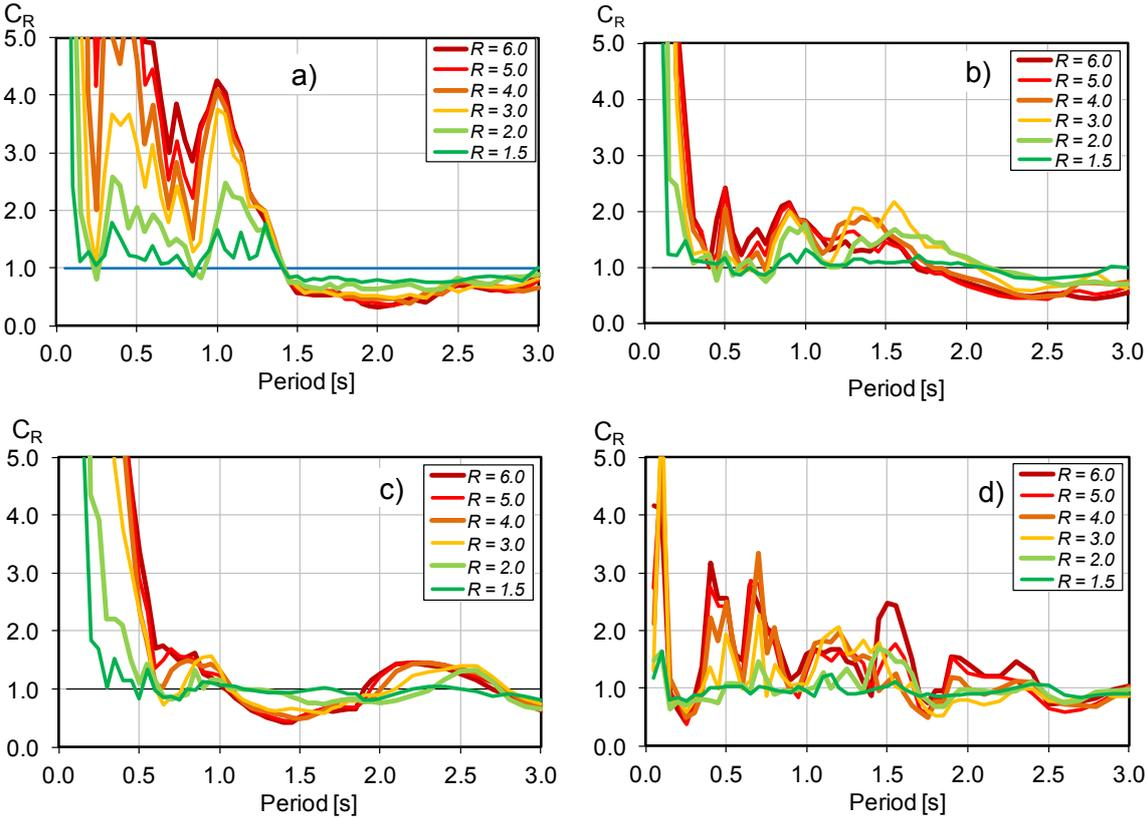
**Figure 5.5.** Inelastic displacement spectra for selected EQGMs: a) CON-L (2010 Chile earthquake), b) CCCC-N64E (2010 Darfield earthquake), c) CCCC-N64E (2010 Christchurch earthquake), and d) MYG-004 (2011 Tohoku earthquake)
