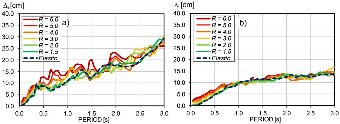
**Figure 5.3.** Inelastic displacement spectra for the selected earthquake ground motions ( $R=3$ )
