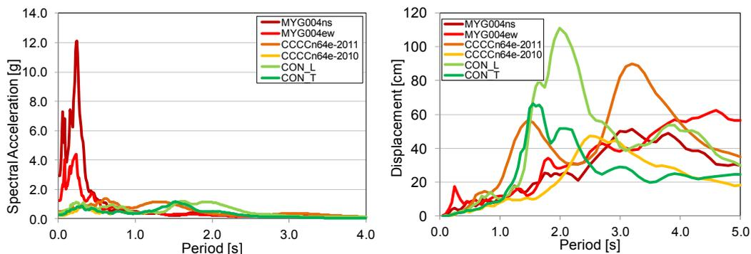
**Figure 3.3** Comparison of 5% damped elastic response spectra computed from EQGMs recorded during the last four most damaging earthquakes: a) Acceleration response spectra, b) displacement response spectra.
