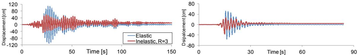
**Figure 5.1.** Comparison of elastic and inelastic displacement time-history ( $R=3$ ) computed from two EQGMs: (a) Concepción (CON) station; (b) Christchurch Cathedral (CCCC) station.
