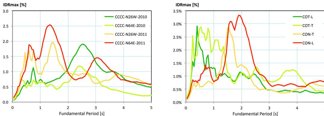
**Figure 4.1.** Generalized Interstory Drift Spectra (GIDS) computed for EQGMs recorded in the 2010 Darfield and 2011 Christchurch earthquakes (on the left) and for EQGMs recorded during the 2010 Maule, Chile (on the right).
