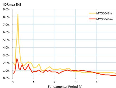
**Figure 4.2.** Generalized Interstory Drift Spectra (GIDS) computed for EQGMs recorded in the city of Miyagi during the 2011 Tohoku earthquake.
