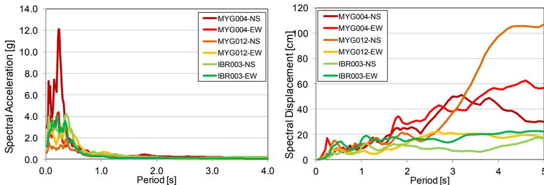
**Figure 3.2** Comparison of elastic response spectra computed from six EQGMs having two distinct waveform sub-events recorded during the 2011 Tohoku earthquake: (a) Acceleration response spectra; (b) Displacement response spectra.
