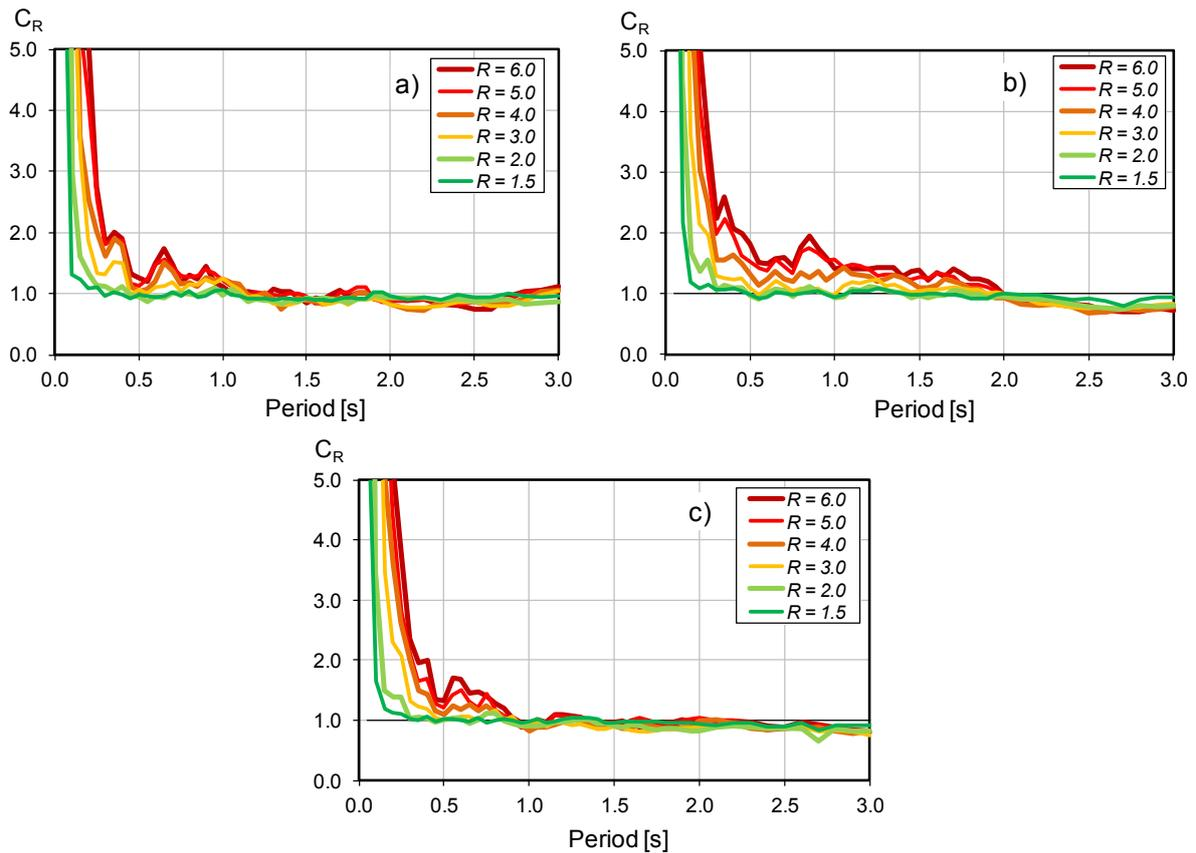
**Figure 5.6.** Median inelastic displacement spectra for three sets of EQGMs recorded in: (a) 38 records from the 2010 Chile earthquake; (b) 34 records from the 2010 Darfield earthquake; and (c) 34 records from the 2011 Christchurch earthquake
