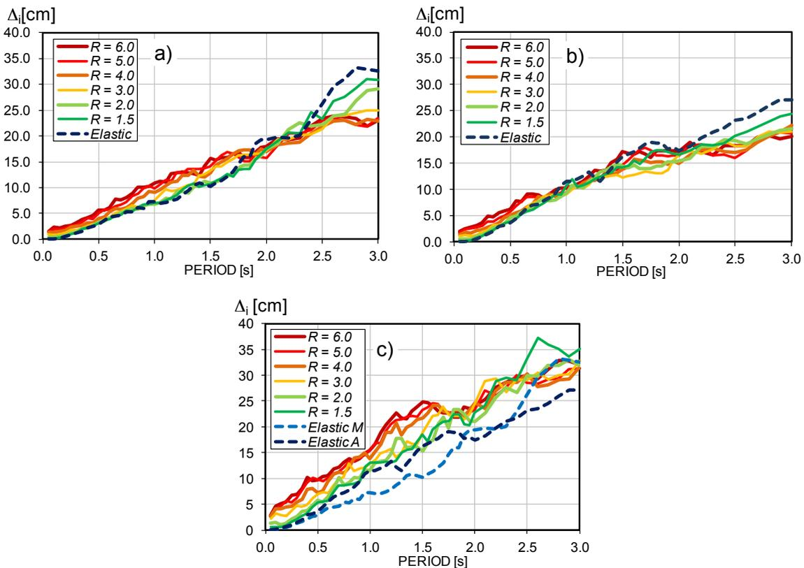
**Figure 5.4.** Peak inelastic displacement demand spectra for sets of EQGMs recorded in: a) 2010 Darfield earthquake, b) 2011 Christchurch earthquake, and c) sequence 2010/2011
