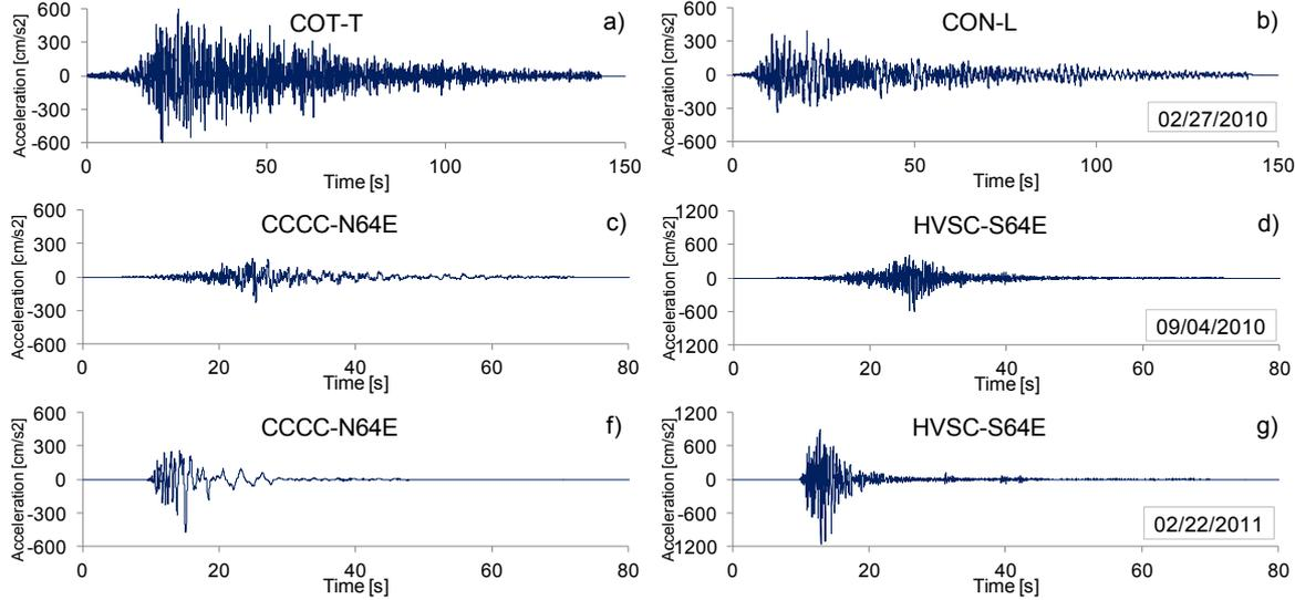
**Figure 2.2** EQGMs recorded during the 2010 Chile earthquake, the 2010 Darfield earthquake, and the 2011 Christchurch earthquake: a) Constitución station (Comp. T), b) Concepción station (comp. L), c) Christchurch Cathedral station (N64E), d) Heathcote Valley Primary School station (comp.S64E), e) Christchurch Cathedral station (N64E), d) Heathcote Valley Primary School station (comp.S64E).
