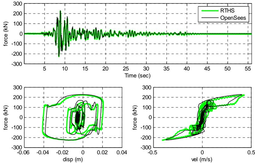
**Figure 6.3.** Comparison of the 3<sup>rd</sup> story MR damper response (Duzce ground motion; LQR Control)
