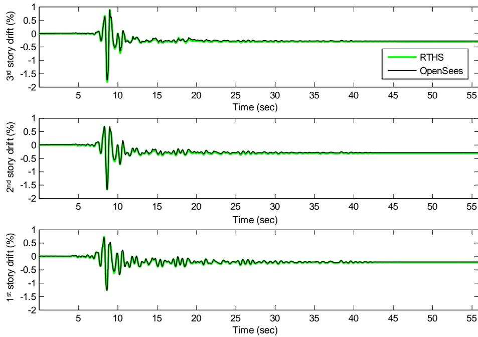
**Figure 6.1.** Comparison of story drifts between RTHS and OpenSees; Duzce EQ ground motion, LQR control
