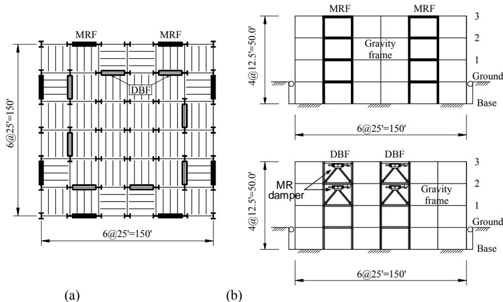
**Figure 2.1.** Prototype 3-story building structure for real-time hybrid simulations: (a) floor plan; (b) elevation
