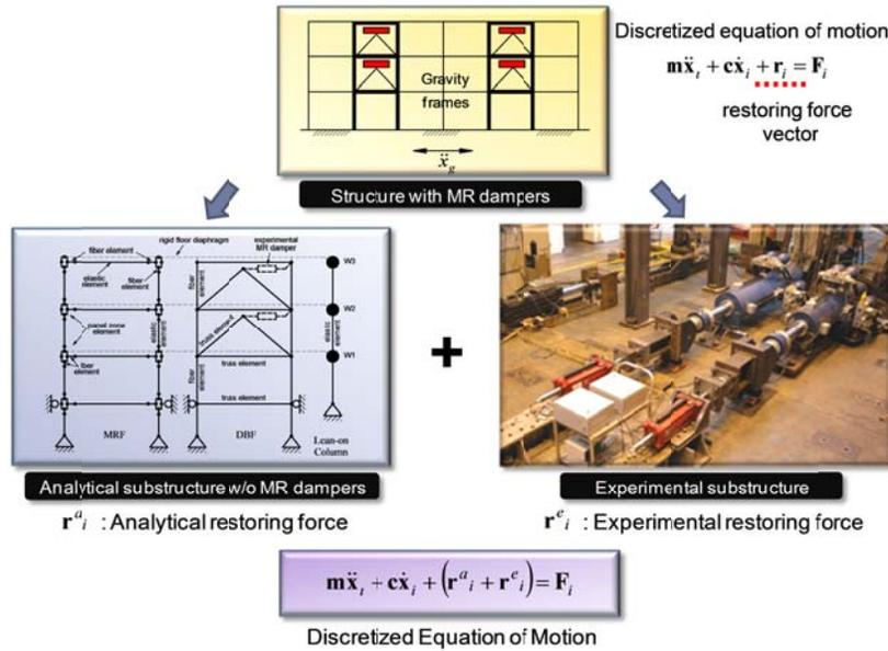
**Figure 3.1.** Schematic of real-time hybrid simulation for a structure with MR dampers: analytical and experimental substructures
