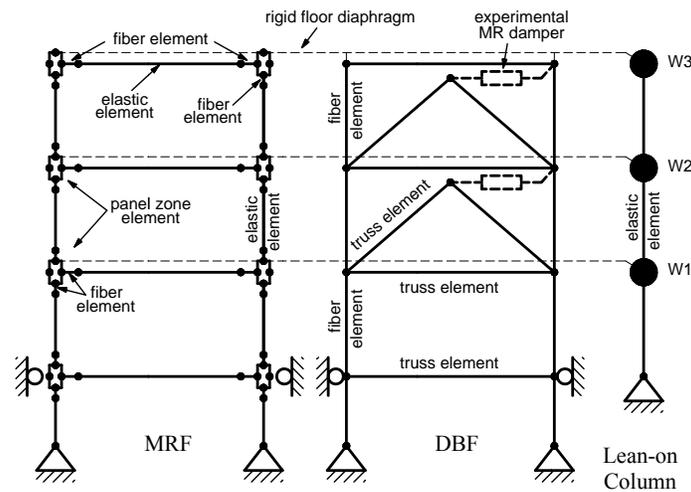
**Figure 3.2.** Analytical substructure model for real-time hybrid simulations (dampers of experimental substructure indicated for clarity)
