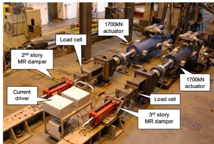
**Figure 3.3.** Experimental substructure with two MR dampers
