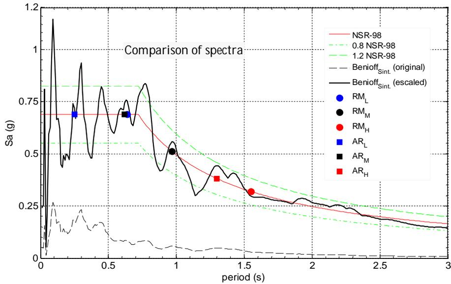
**Figure 5.2.** Original Synthetic-Benioff accelerogram and band-scaled accelerogram response spectra. For both cases 80% and 120% limits of design spectra were drawn.
