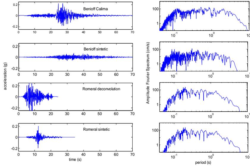
**Figure 4.4.** Recommended accelerograms by the micro-zoning seismic study for Manizales for be used in dynamical analyses. For easy comparison all the graphics have the same scale.
