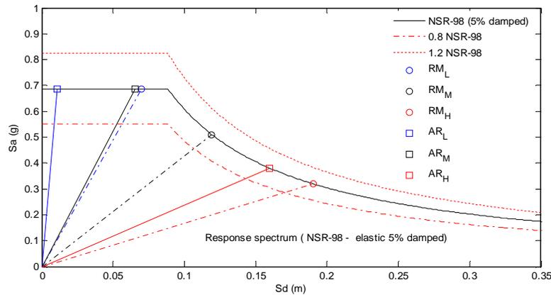
**Figure 4.3.** Design spectrum for the location of the studied buildings in Manizales in ADRS format.
