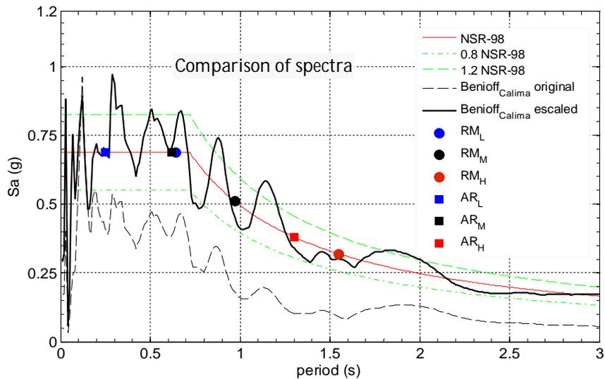
**Figure 5.1.** Original Calima-Benioff accelerogram and band-scaled accelerogram response spectra. For both cases 80% and 120% limits of design spectra were drawn.
