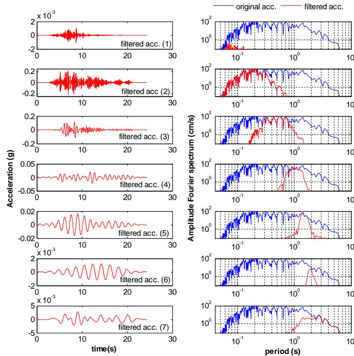
**Figure 4.5.** Accelerograms resulting from applying filters, based on limit frequencies of Table 4.1, to Romeral-deconvolution accelerogram included in Fig. 4.4. To the left seven signals in time domain are displayed; to the right seven response spectra in period domain, aside the amplitude Fourier spectrum for original accelerogram
