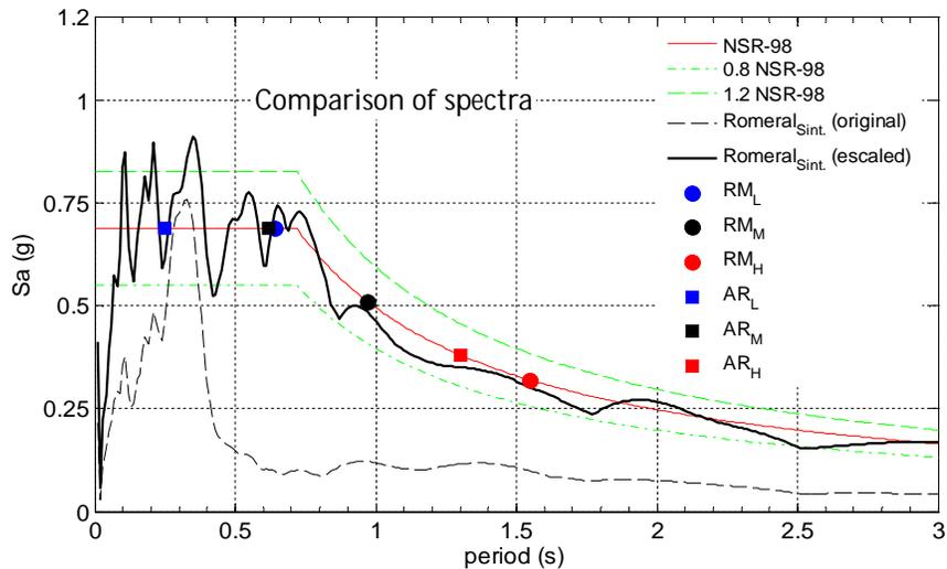
**Figure 5.3.** Original Synthetic-Romeral accelerogram and band-scaled accelerogram response spectra. For both cases 80% and 120% limits of design spectra were drawn.
