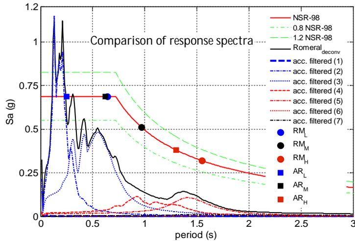
**Figure 4.6.** Response spectra of both original accelerogram and seven accelerograms from Fig. 4.5.
