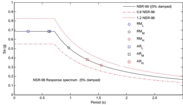
**Figure 4.2.** Design spectrum for the location site of the studied buildings in Manizales. It has been taken  $A_a=0.25g$ ,  $I=1.1$ , corresponding to educational buildings, and  $S=1.5$  corresponding to a soil type 3.
