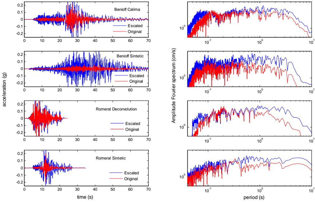
**Figure 5.4.** Accelerograms scaling equal to original.
