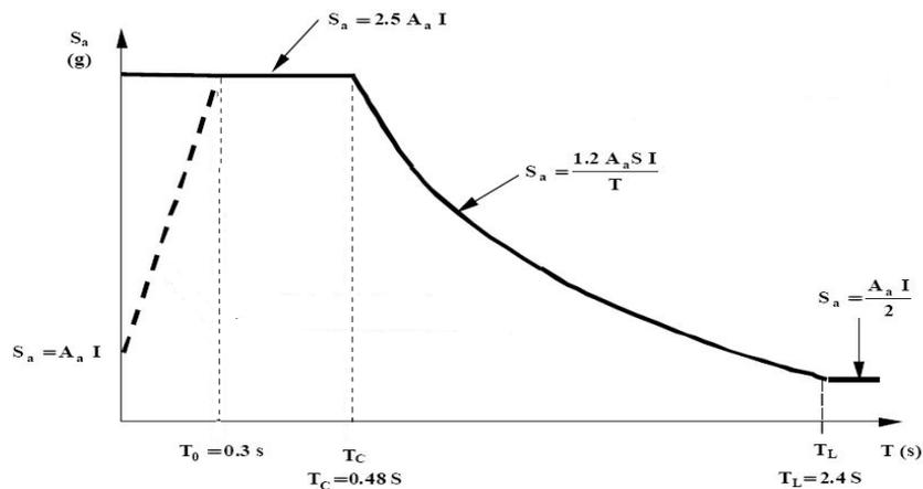
**Figure 4.1.** Elastic response spectrum 5% damped
