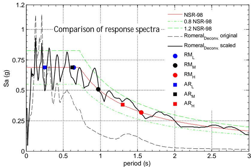
**Figure 4.7.** Original accelerogram and band-scaled accelerogram response spectra. For both cases 80% and 120% limits of design spectra were drawn.
