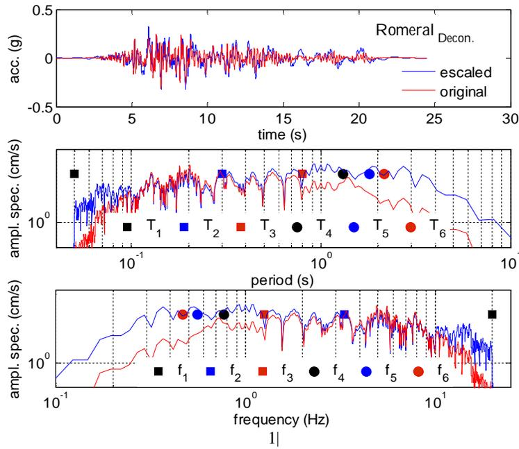
**Figure 4.8.** Original and scaled accelerograms. Up: Time domain. Down: Fourier amplitude spectra for period and frequency domains. Also periods and frequencies of Table 4.1 are displayed.
