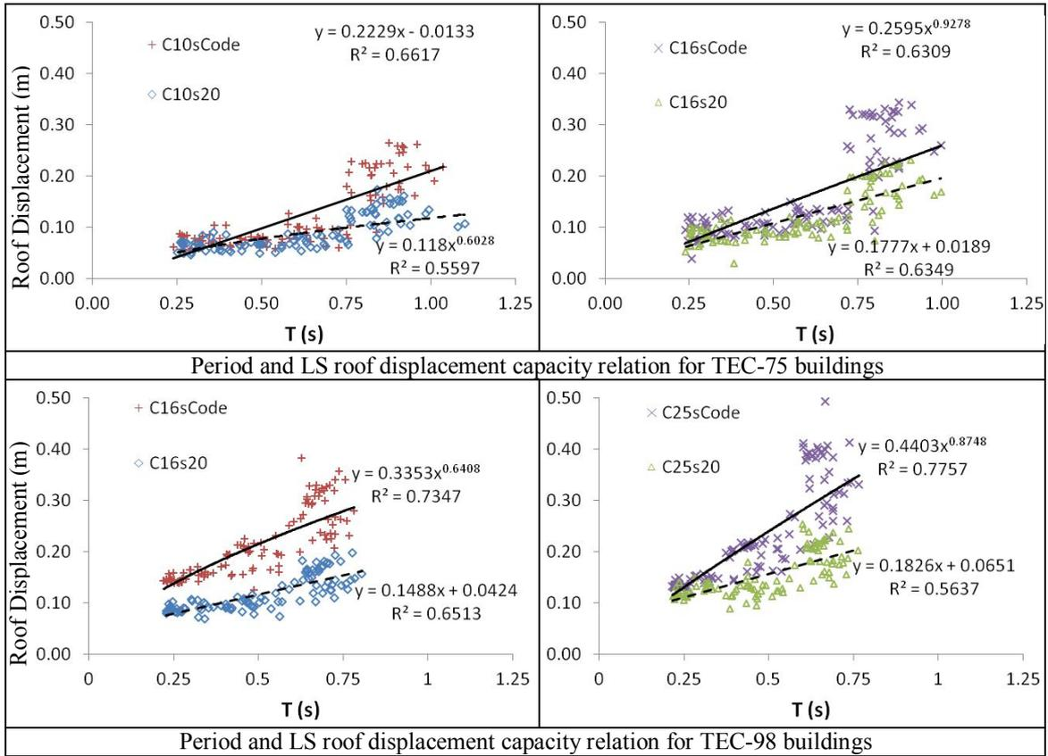
Figure 4.2. Period and LS roof displacement capacity relation for TEC-75 and TEC-98 buildings
