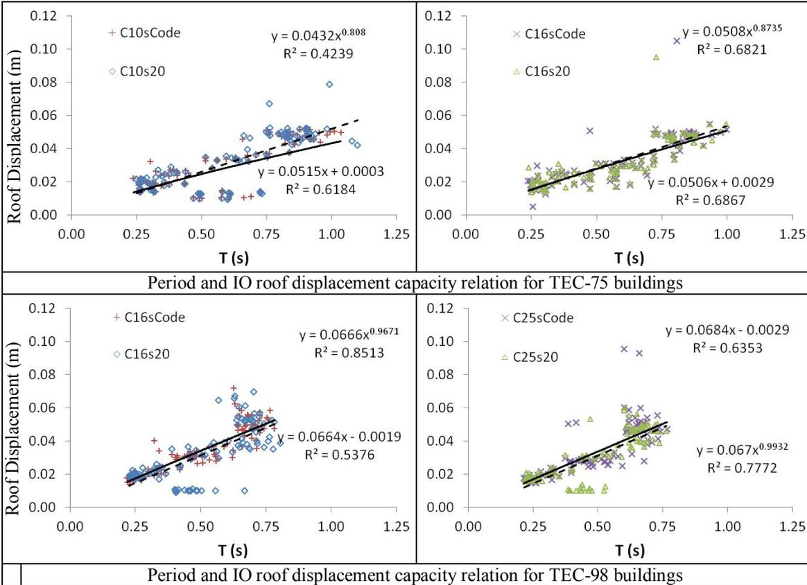
Figure 4.1. Period and IO roof displacement capacity relation for TEC-75 and TEC-98 buildings
