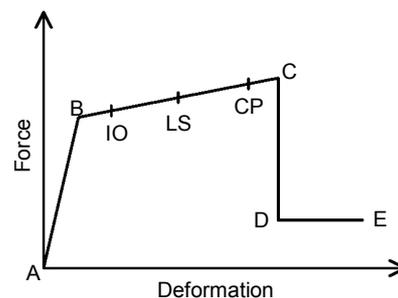
**Figure 2.2.** Force-Deformation relationship of a typical plastic hinge
