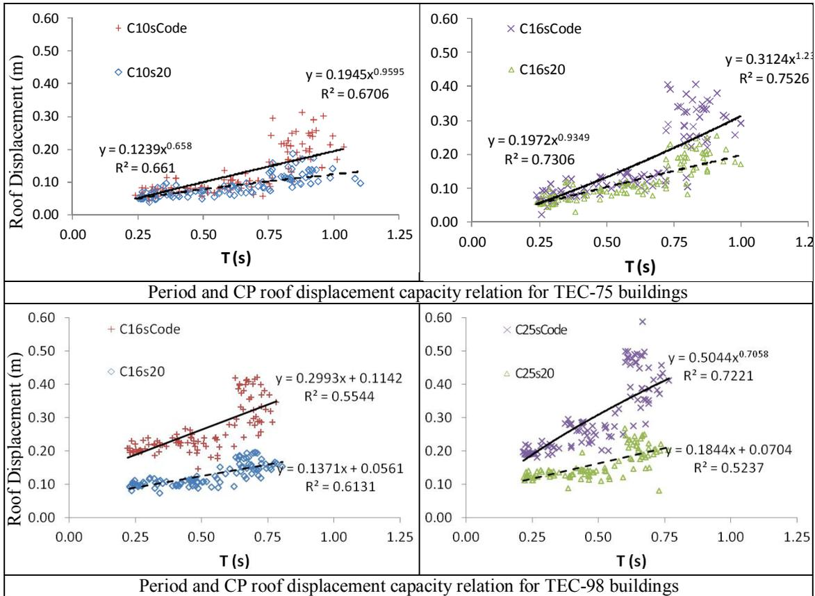
Figure 4.3. Period and CP roof displacement capacity relation for TEC-75 and TEC-98 buildings
