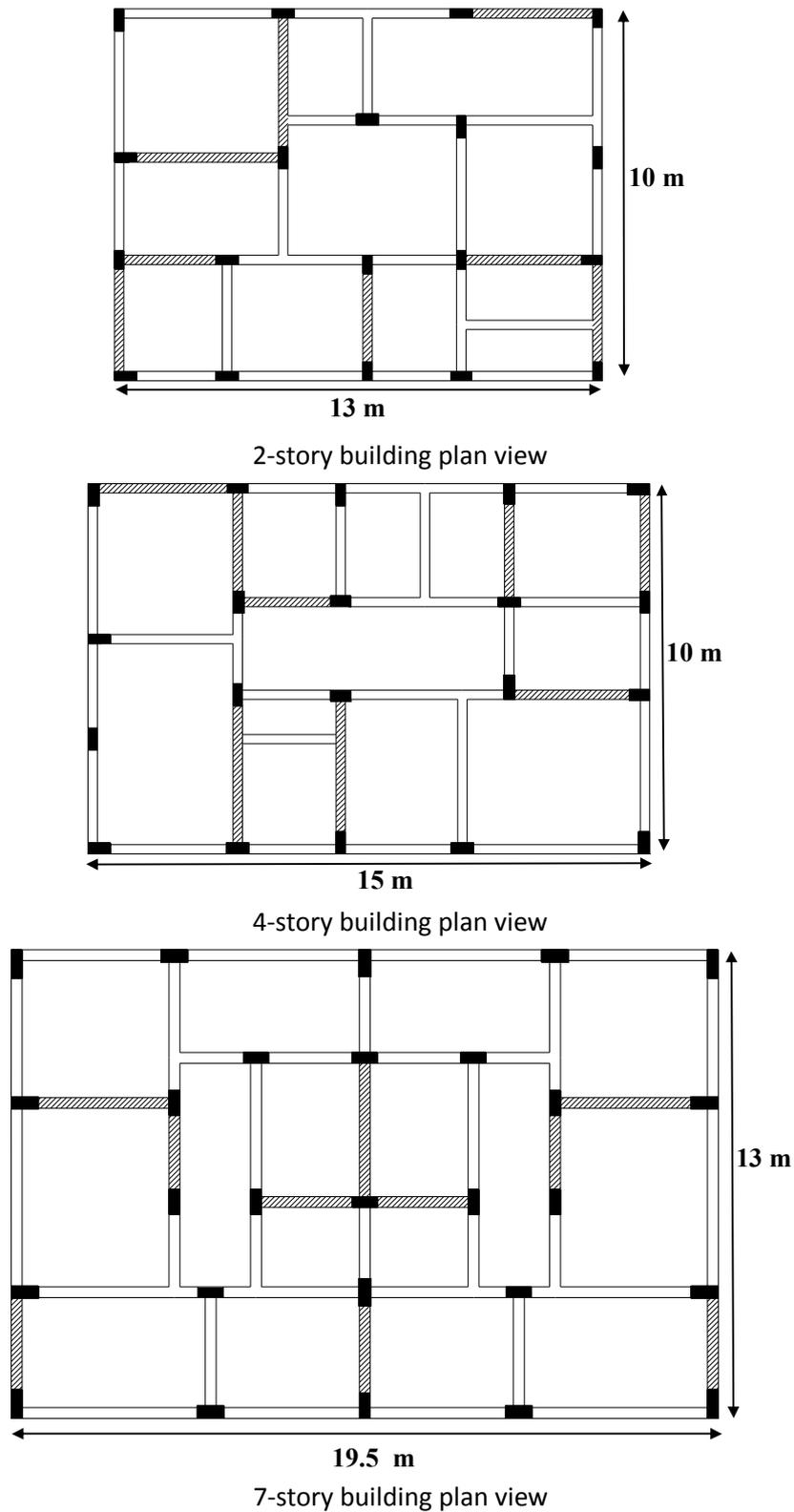
**Figure 2.1.** Plan view of the considered buildings (load carrying infill-walls are shaded)
