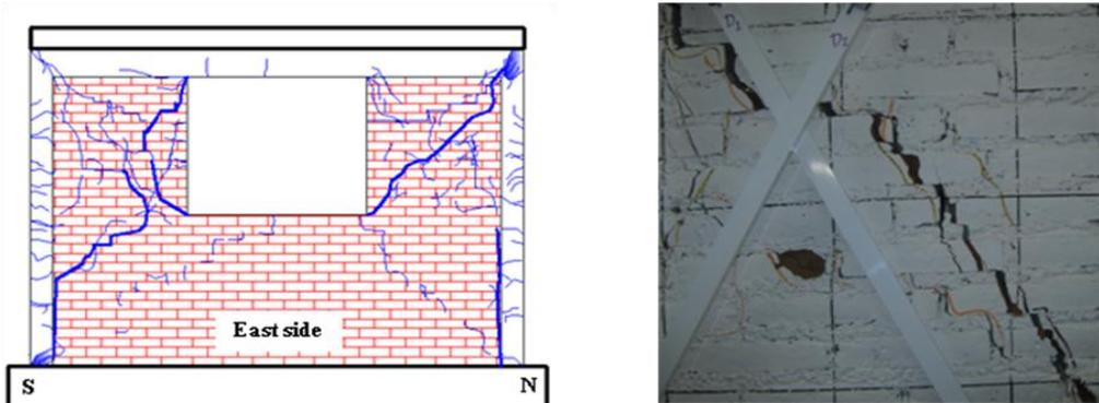
**Figure 5.2.** Crack pattern for the East Side and damage due to a diagonal crack
