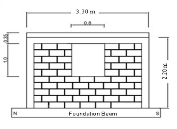
**Figure 3.2.** Block wall specimen with overall dimensions
