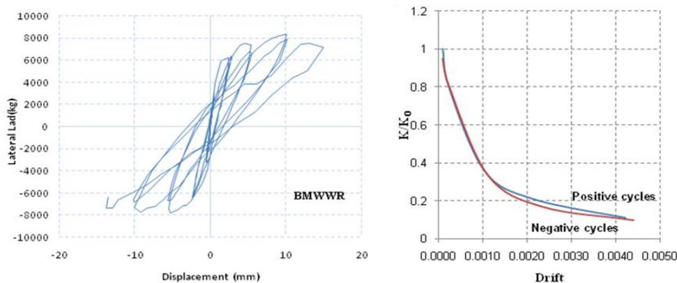
**Figure 5.3.** Hysteretic curve and normalized stiffness degradation curve for Wall BMWWR
