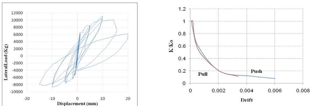
**Figure 5.5.** Hysteretic curve and normalized stiffness degradation curve for Wall BMWRV
