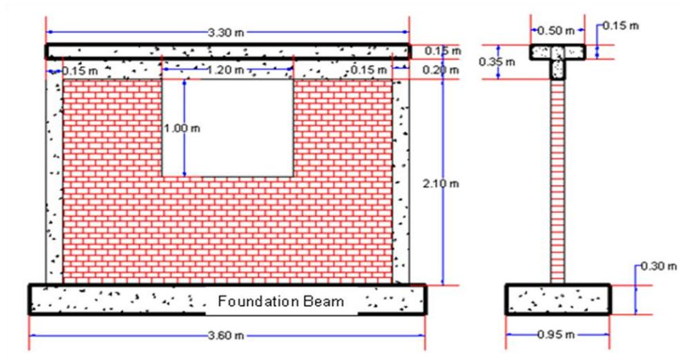
Figure 3.1. Brick wall specimen with overall dimensions
