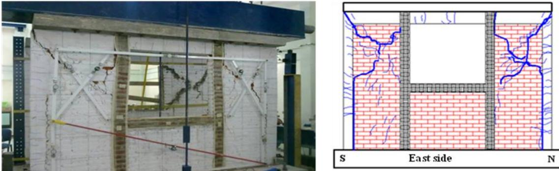
**Figure 5.4.** Damage due to a diagonal crack and crack pattern for the East Side
