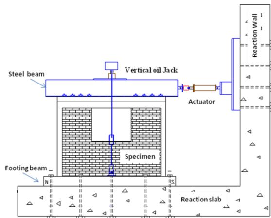
**Figure 4.1.** Test set up
