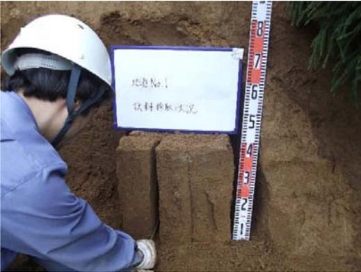
Figure 2.6. Sampling of undisturbed block of clayey loam in the cliff
