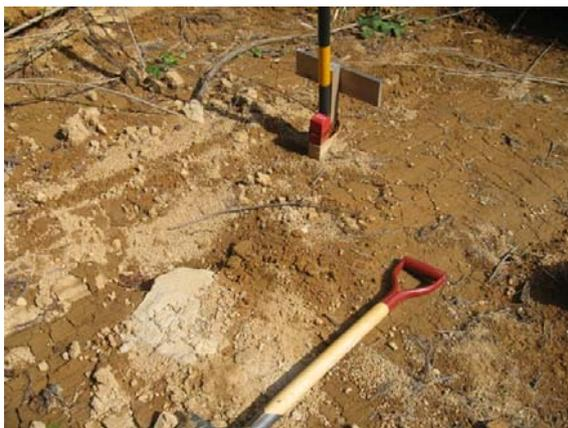
**Figure 2.3.** Exposed planar slip surface with clayey loam including a lot of small stone pieces
