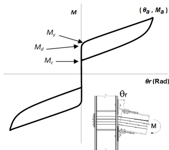
**Figure 2.3.** Moment-relative rotation curve of the connecting post-tensioned
