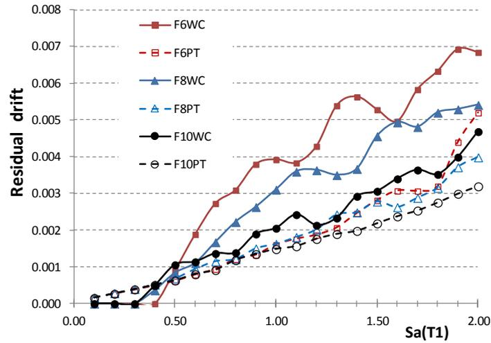
Figure 4.6. Residual drift of the frames FWC and FPT
