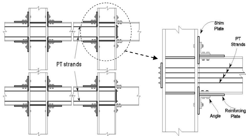
**Figure 2.2.** Angles and post-tensioned strands in FPT
