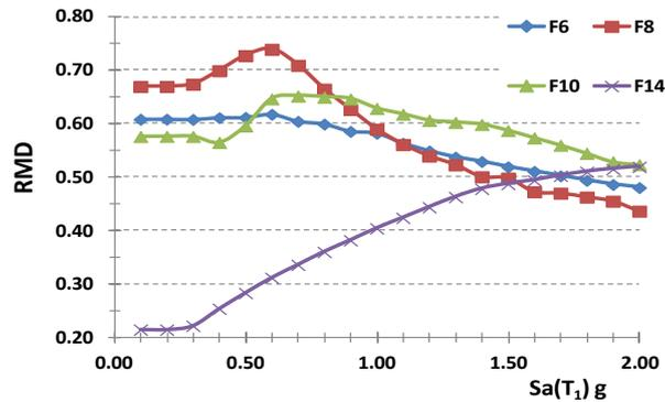
Figure 4.3. Ratio of maximum inter-story drift between FPT and FWC
