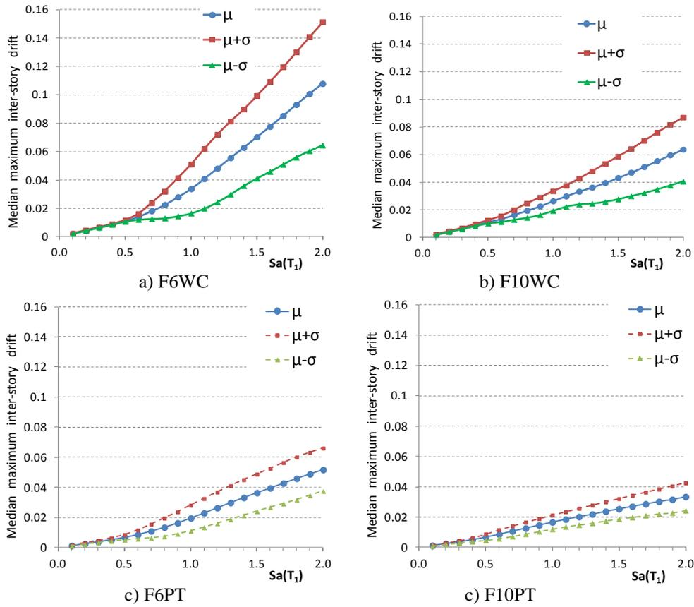
Figure 4.1. Drift maximum median and standard deviation for FWC and FPT
