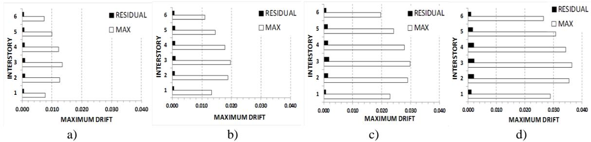
Figure 4.4. Maximum interstory drift F6PT for: a) 0.8g, b) 1.0g, c) 1.2g and d) 1.5g
