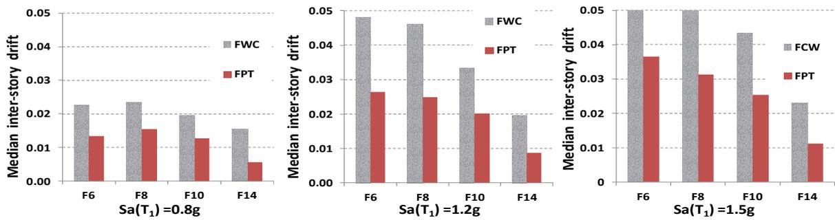
Figure 4.2. Median maximum drift of the frames FWC and FPT
