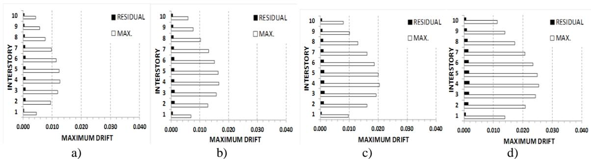
Figure 4.5. Maximum interstory drift F10PT for: a) 0.8g, b) 1.0g, c) 1.2g and d) 1.5g
