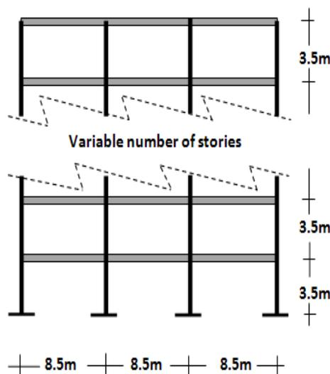
**Figure 2.1.** Overall dimensions the frames
