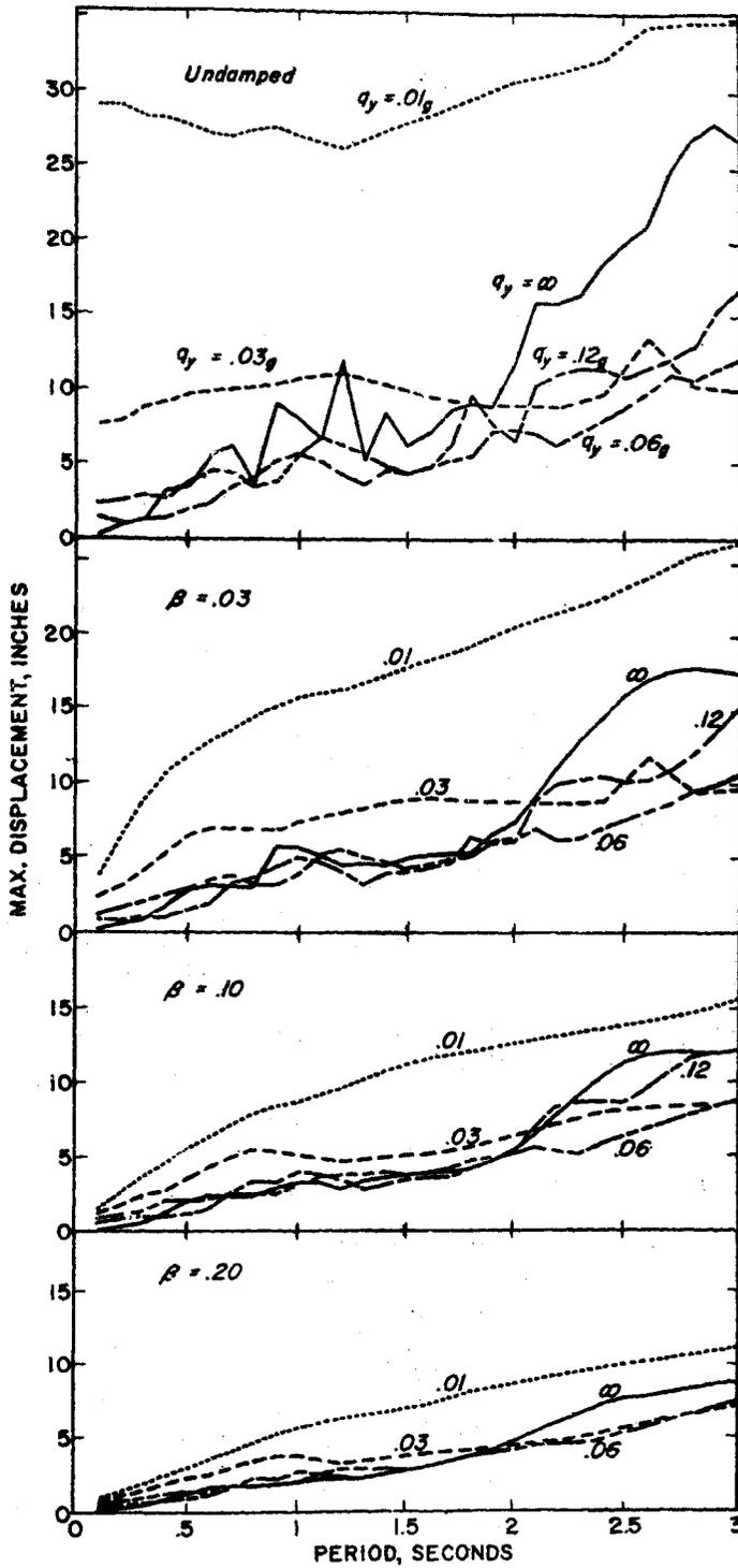
Fig. 5. Displacement spectrum (N-S component, El Centro, California, earthquake of May 18, 1940).
