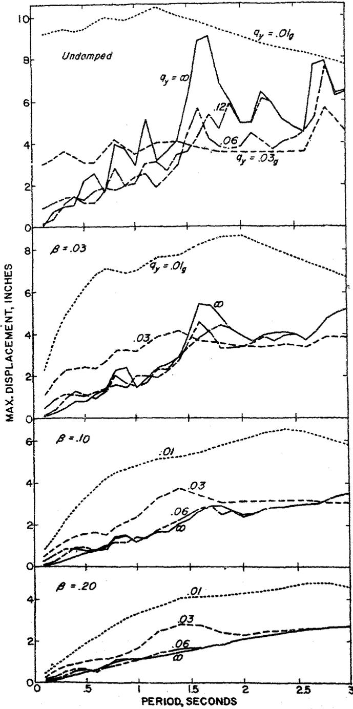
Fig. 6. Displacement spectrum (N69°W component, Taft, California, earthquake of July 21, 1952).
