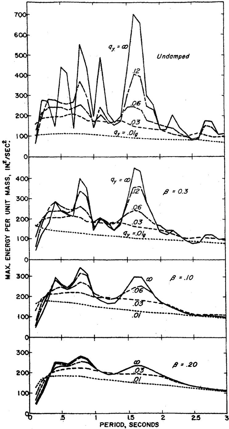
Fig. 4. Energy input spectrum (N69°W component, Taft, California, earthquake of July 21, 1952).
