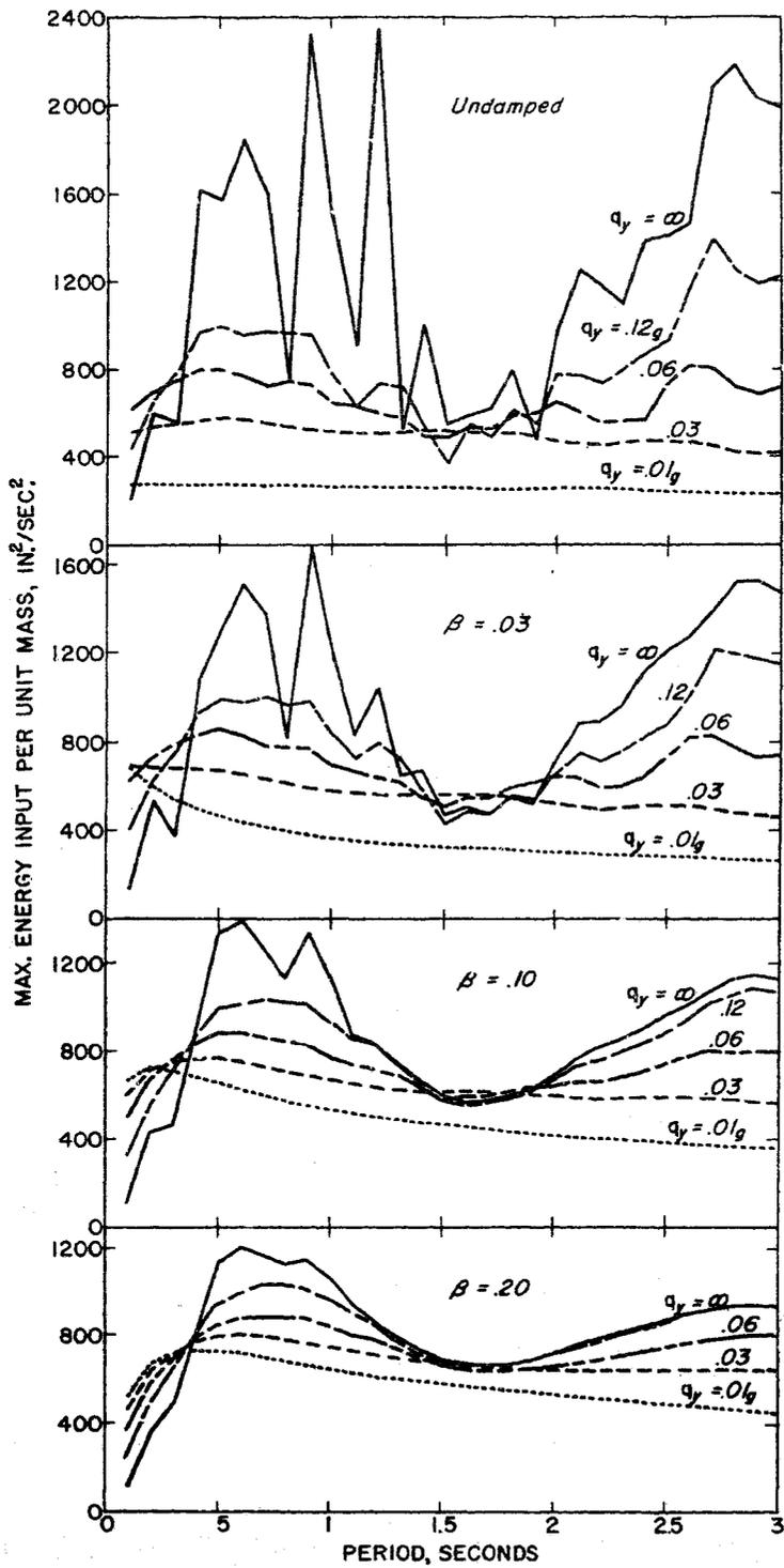
Fig. 3. Energy input spectrum (N-S component, El Centro, California, earthquake of May 18, 1940).
